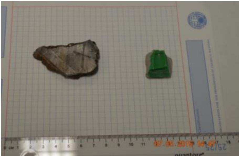
**FIGURE 3: METAL FRAGMENT OF SAMPLE 08 SDS-01, SHOWING 45° DEGREE ANGLE EDGE**
