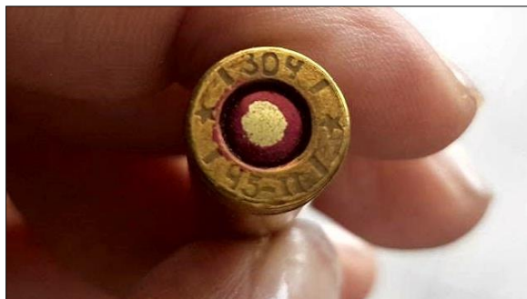
Figure 5: 7.62x25 mm round manufactured at Kouskovo – 304 factory in the former Soviet Union.
