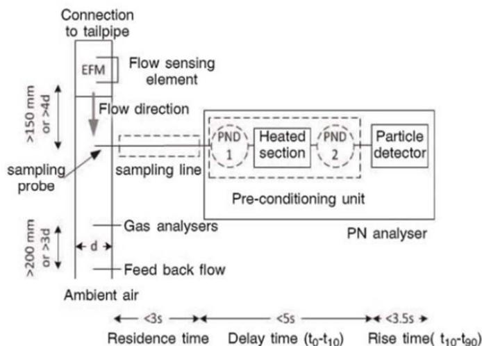
The PN analyser shall be connected to the sampling point via a sampling probe which extracts a sample from the centreline of the tailpipe tube. As specified in paragraph 3.5. of Annex 4, if particles are not diluted at the tailpipe, the sampling line shall be heated to a minimum temperature of 373 K (100 °C) until the point of first dilution of the PN analyser or the particle detector of the analyser. The residence time in the sampling line shall be less than 3 s.
