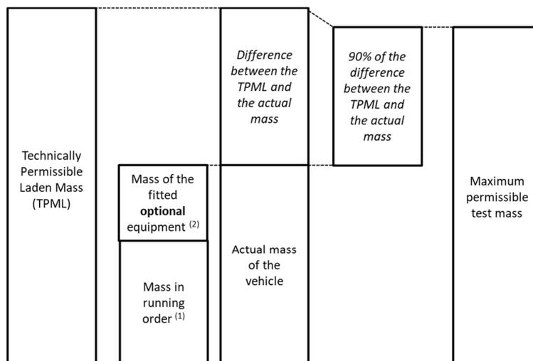
(1) means the mass of the vehicle, with its fuel tank(s) filled to at least 90 per cent of its or their capacity/capacities, including the mass of the driver, fuel and liquids, fitted with the **standard equipment** in accordance with the manufacturer's specifications and, when they are fitted, the mass of the bodywork, the cabin, the coupling and the spare wheel(s) as well as the tools.
