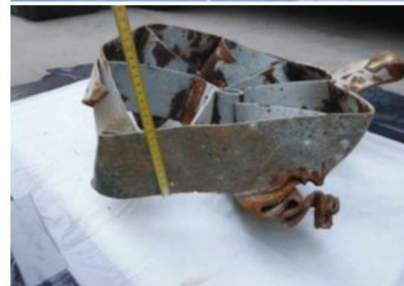
Fragments are from high-explosive bomb. They show traces of severe metal corrosion. According to the photo, the corrosion is aged at least five years.
