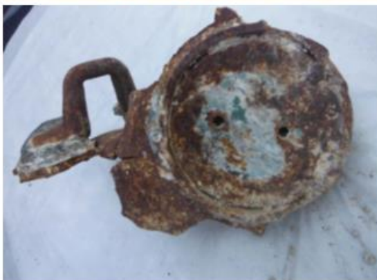
Fragments are from high-explosive bomb. They show traces of severe metal corrosion. According to the photo, the corrosion is aged at least five years.
