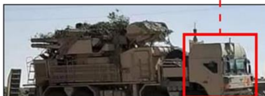
Pantsir S-1 supplied to UAE in Libya on 19 June 2019. NOTE: MAN SX45 Heavy High Mobility Truck as the ground mobility platform. Reported in S/2019/519.
