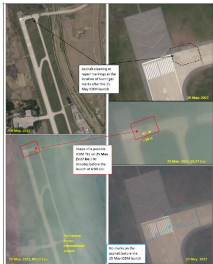
Figure 21: 25 May 2022 (06:00 Loc.) - possible location of the ICBM launch pad at 39°13'14"N 125°39'55"E
