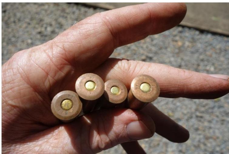
Figure XVII: Sample of 7.62x52Rmm ammunition
