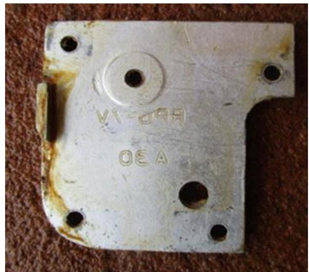
Rear view of the aluminium plate covering the percussion mechanism.
