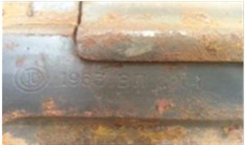
ARM – Manufactured in Bulgaria – Year of manufacture 1963 – Serial number: VP2204
