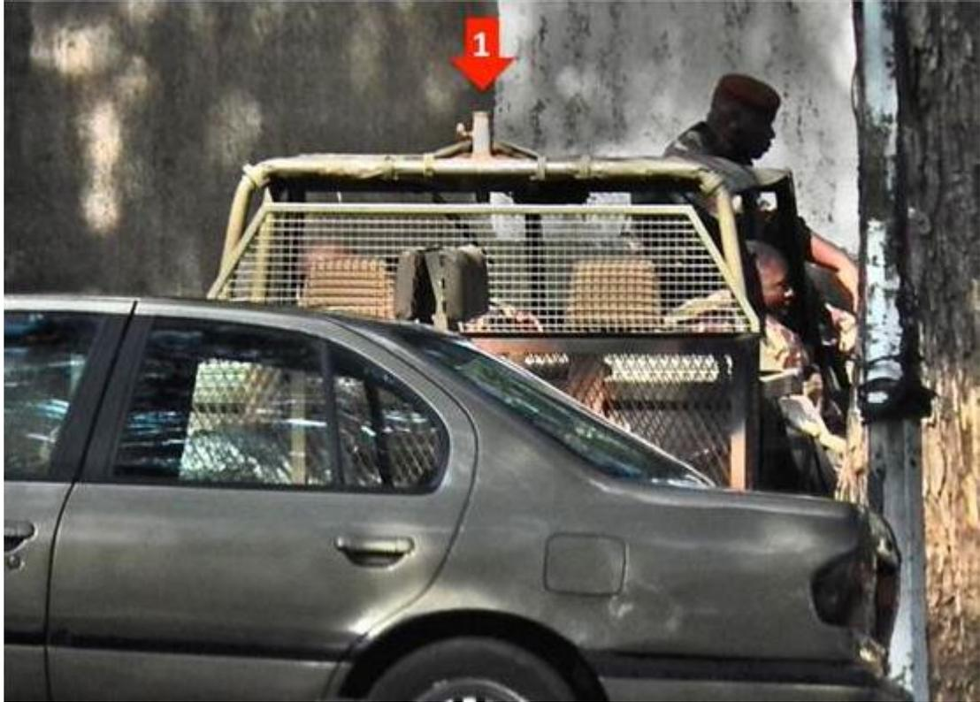
1. Mounting for a heavy machine gun (not mounted).
