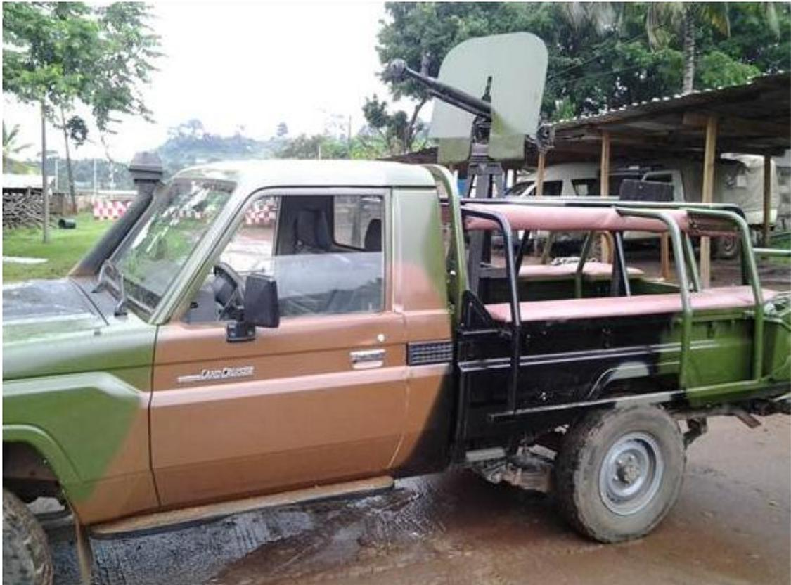
**Mod B: ALTV armed with a 12.7-mm heavy machine gun**
