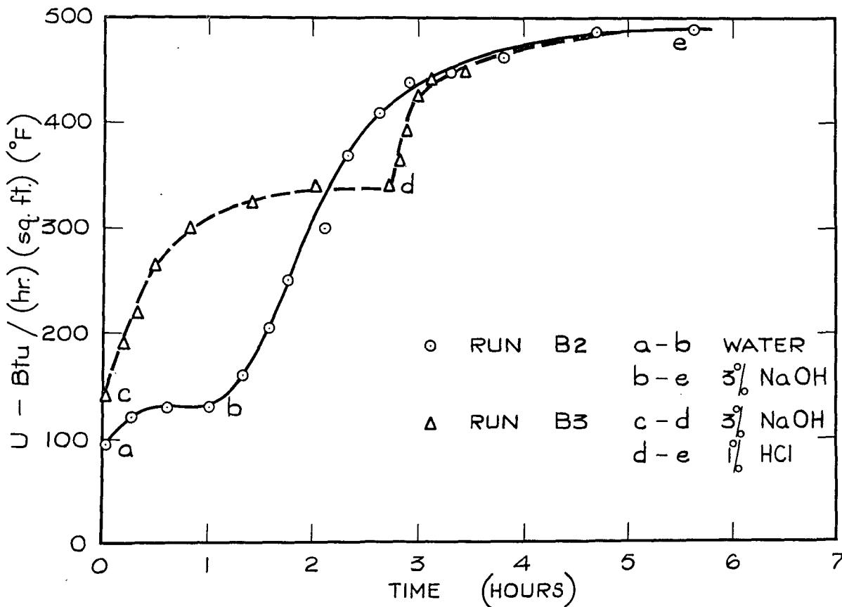
Figure 9. Removal of scale from evaporator tubes
