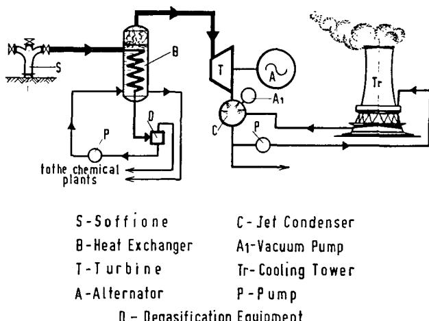
Figure 5. Condensing steam turbine cycle with heat exchanger
