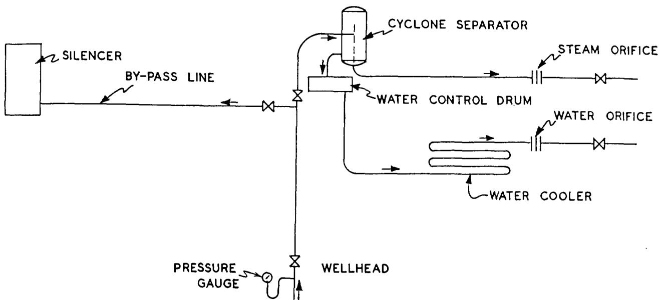
Figure 1. Diagrammatic layout of separating equipment for output testing
