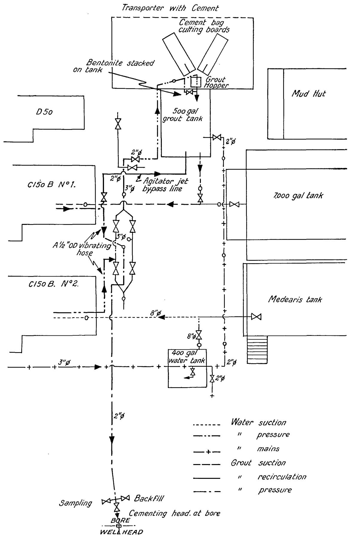
Figure 3. Wairakei geothermal power project. Cementing line layout for 3 000-foot drill
