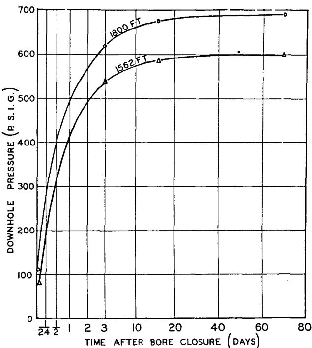
Figure 1. Downhole pressure recovery after a bore closure
