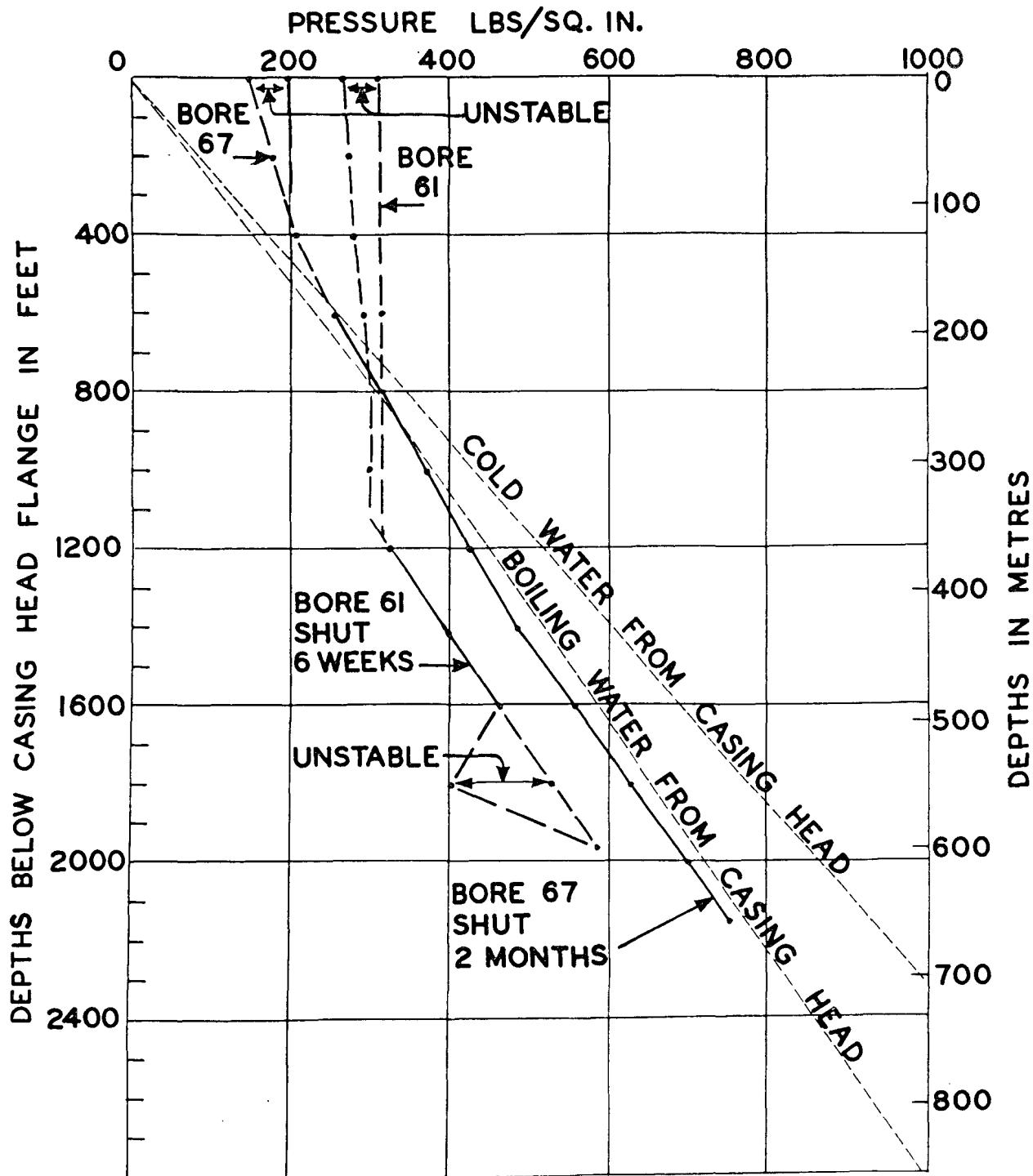
Figure 5. Pressure runs in bores 61 and 67
