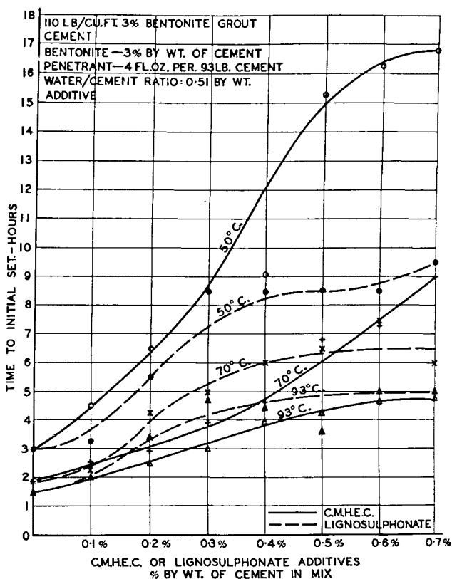
Figure 4. Setting times v. additive proportion for cement/bentonite slurries
