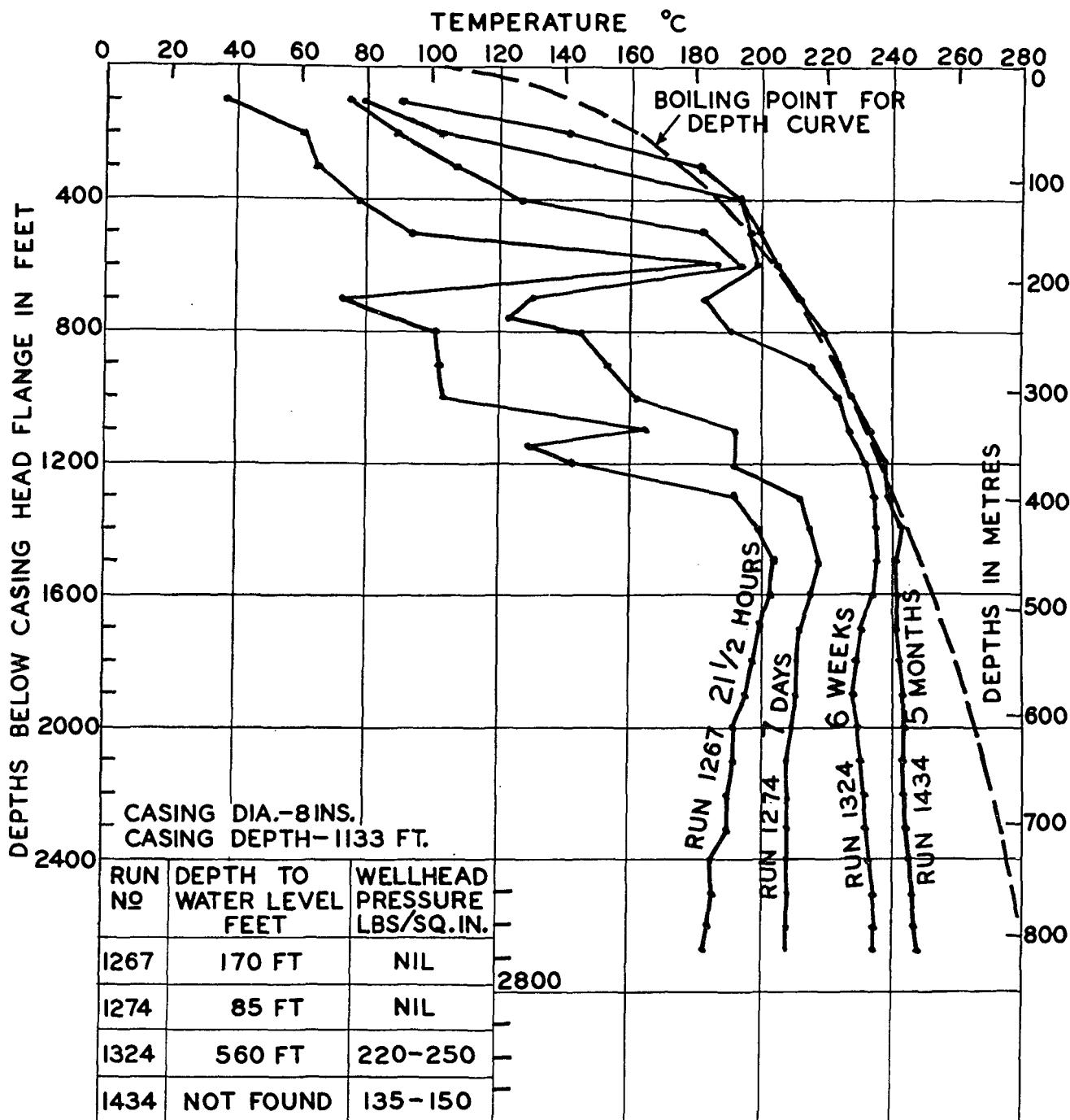
Figure 4. Temperature runs in bore 24 after various standing times
