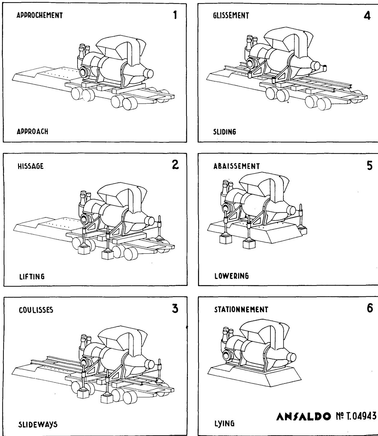
Figure 7. Scheme of assembly operations of a 3 000-3 500 kW turbine-generator set
