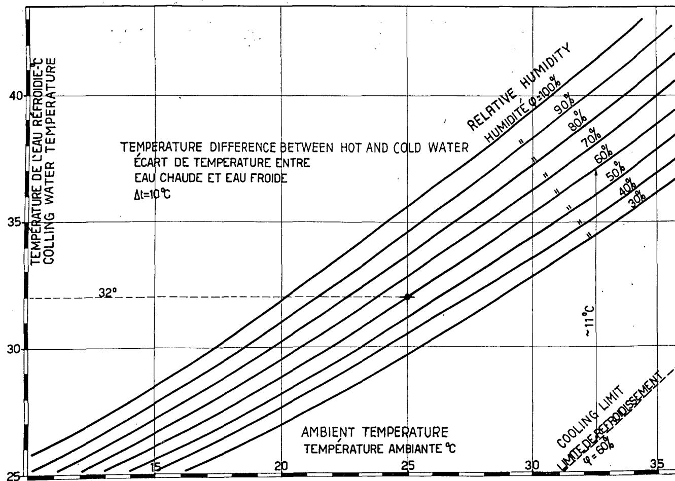
Figure 9. Hyperbolic tower, 9 000 m<sup>3</sup>/h: cooling curves
