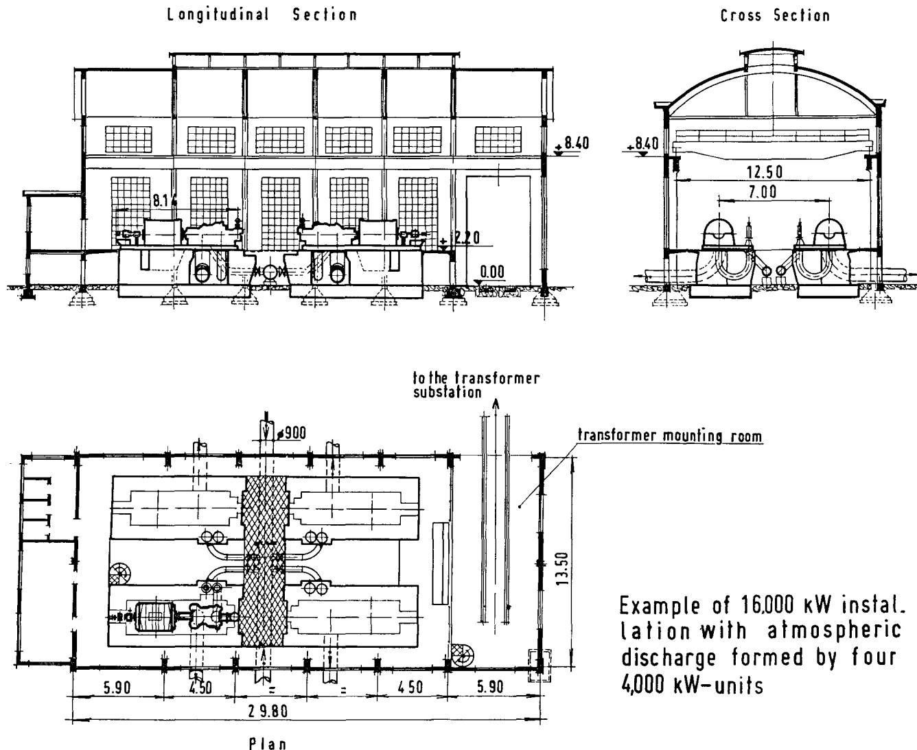
Figure 4. Example of a 16 000 kW installation with atmospheric discharge formed by four 4 000-kW units
