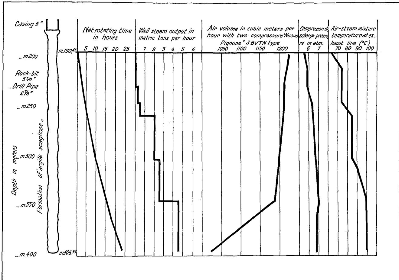
Figure 3. Air drilling in a well producing geothermal steam (air volume requirements/well steam output)
