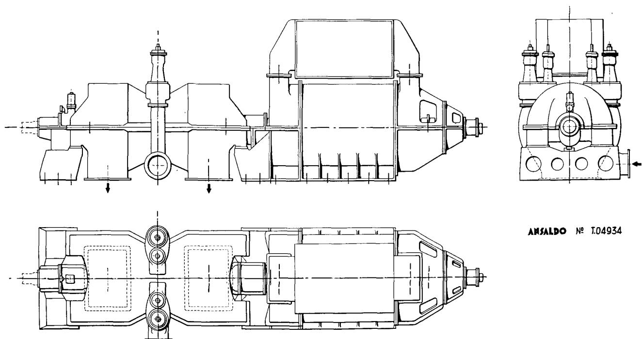
Figure 5. 15 000 kW turbine-generator set
