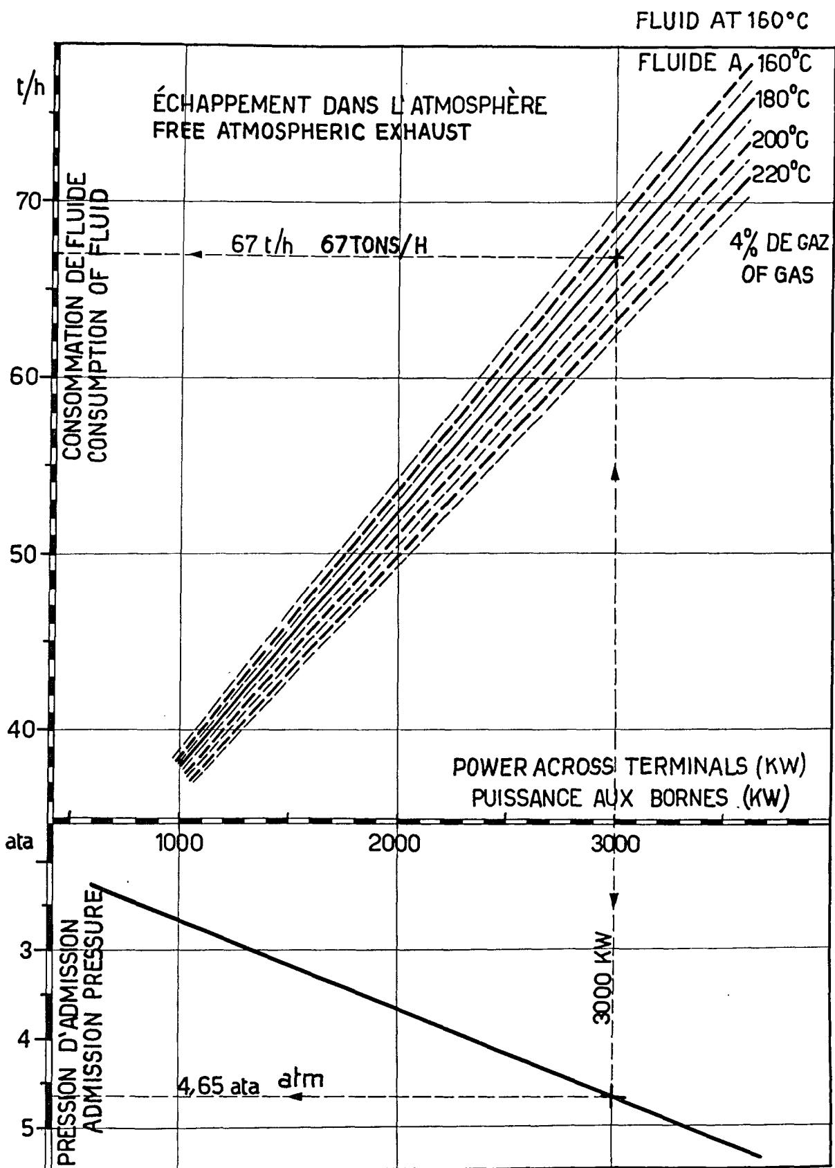
Figure 5. Consumption curves of 5 atm 3 500 kW unit
