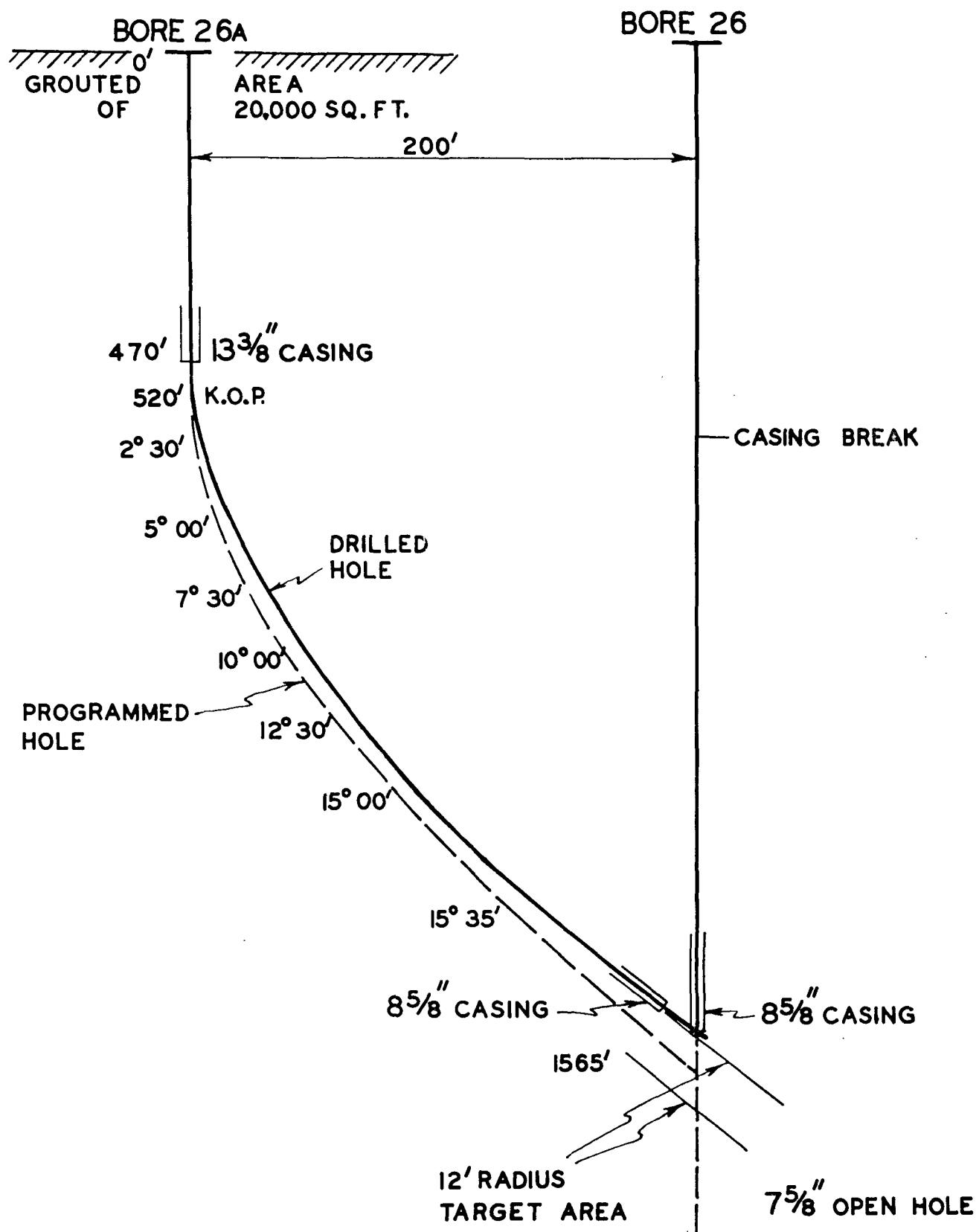
Figure 4. Deviated bore No. 26a
