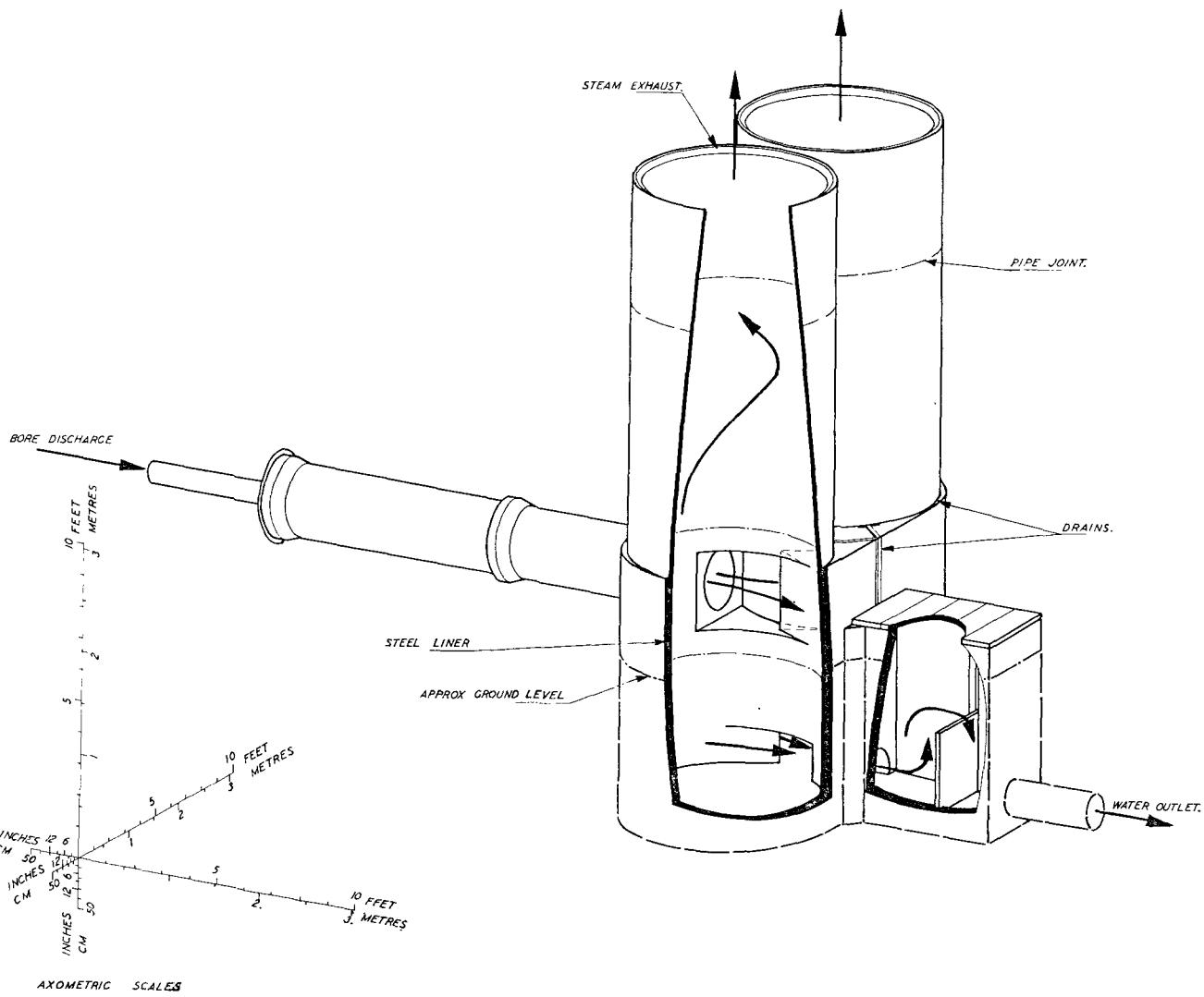
Figure 6. Twin cyclone silencer : cut-away axometric projection
