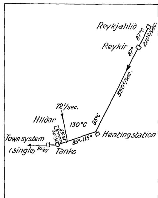
Figure 1. Reykjavik heating system: sketch of main feed-lines
