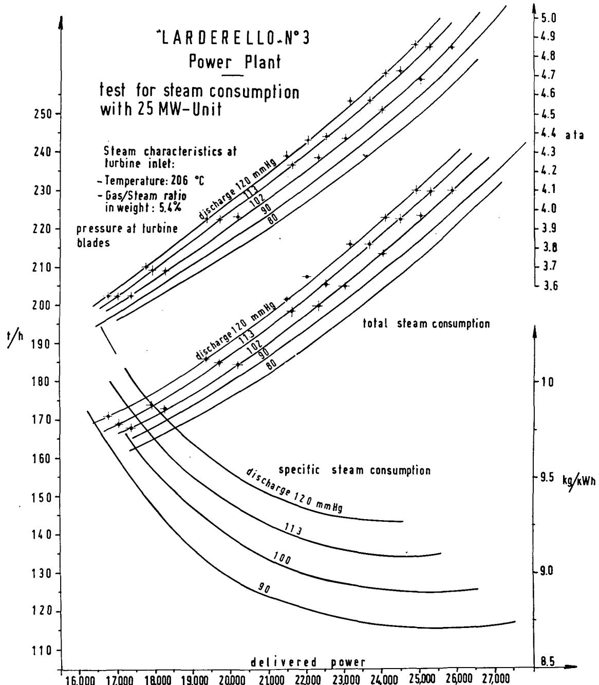
Figure 9. Larderello No. 3 — test for steam consumption with a 25-MW unit
