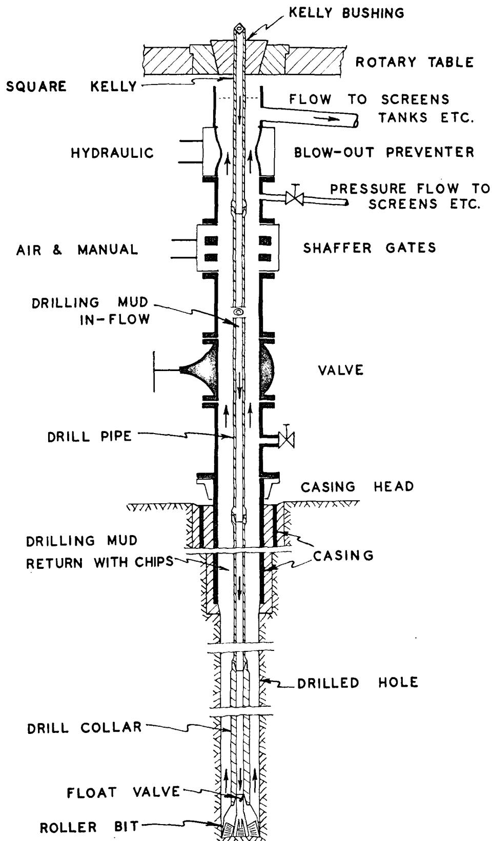
Figure 3. Drilling string and blowout preventer equipment
