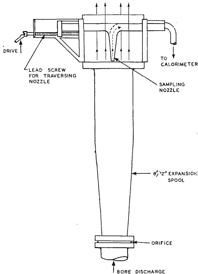
Figure 2. General arrangement of steam sampler
