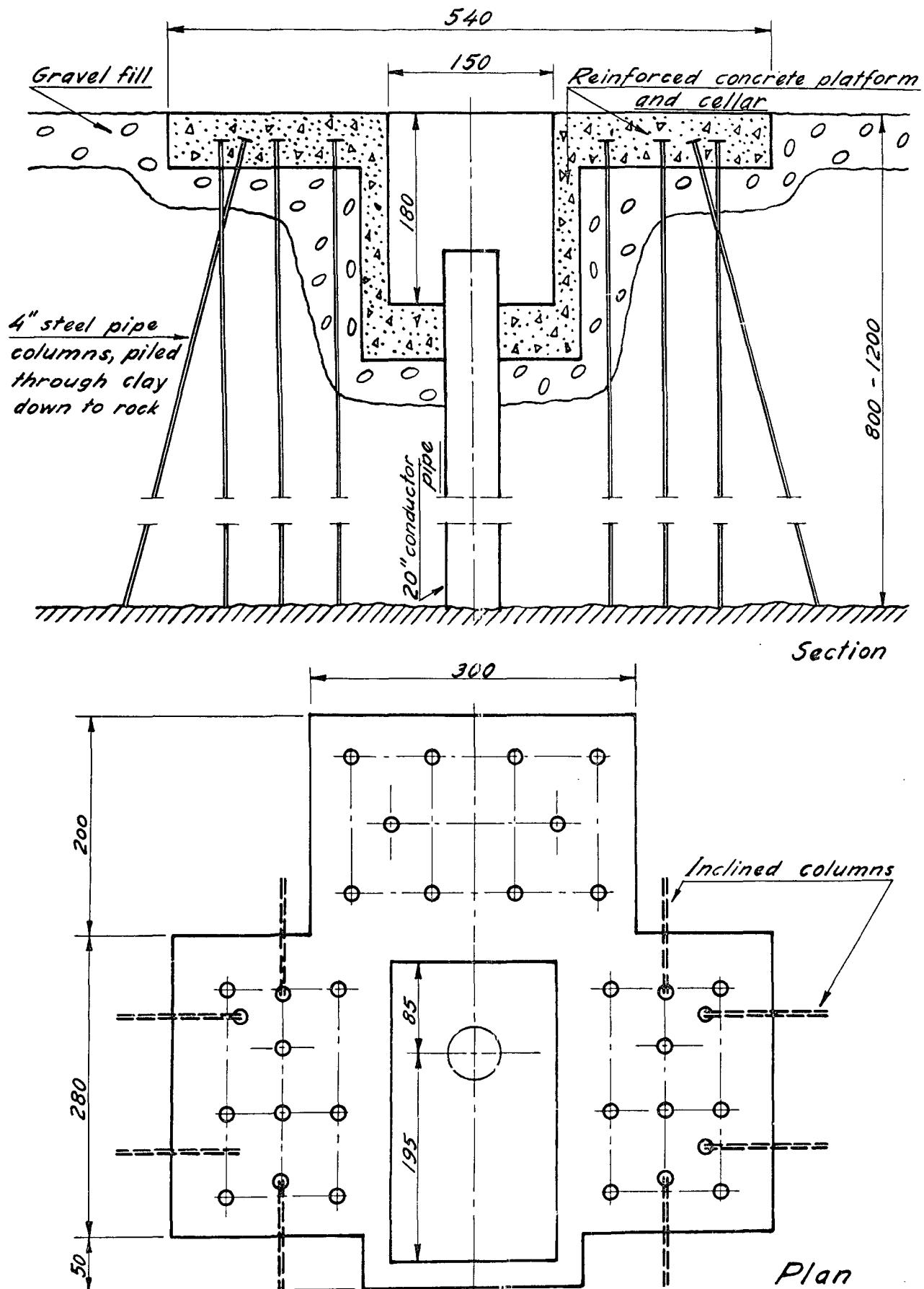
Figure 3. Foundation for rotary drilling equipment at Krysuvik, Iceland
