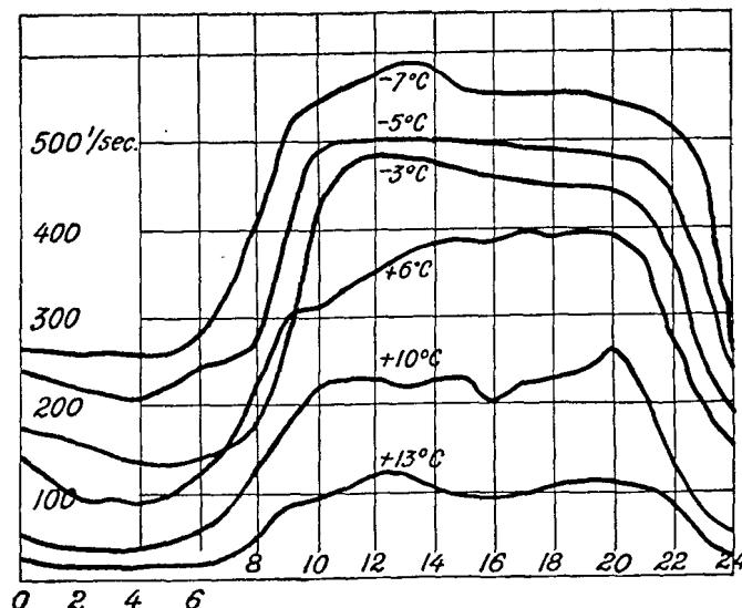
Figure 2. Reykjavik heating system: daily load curve
