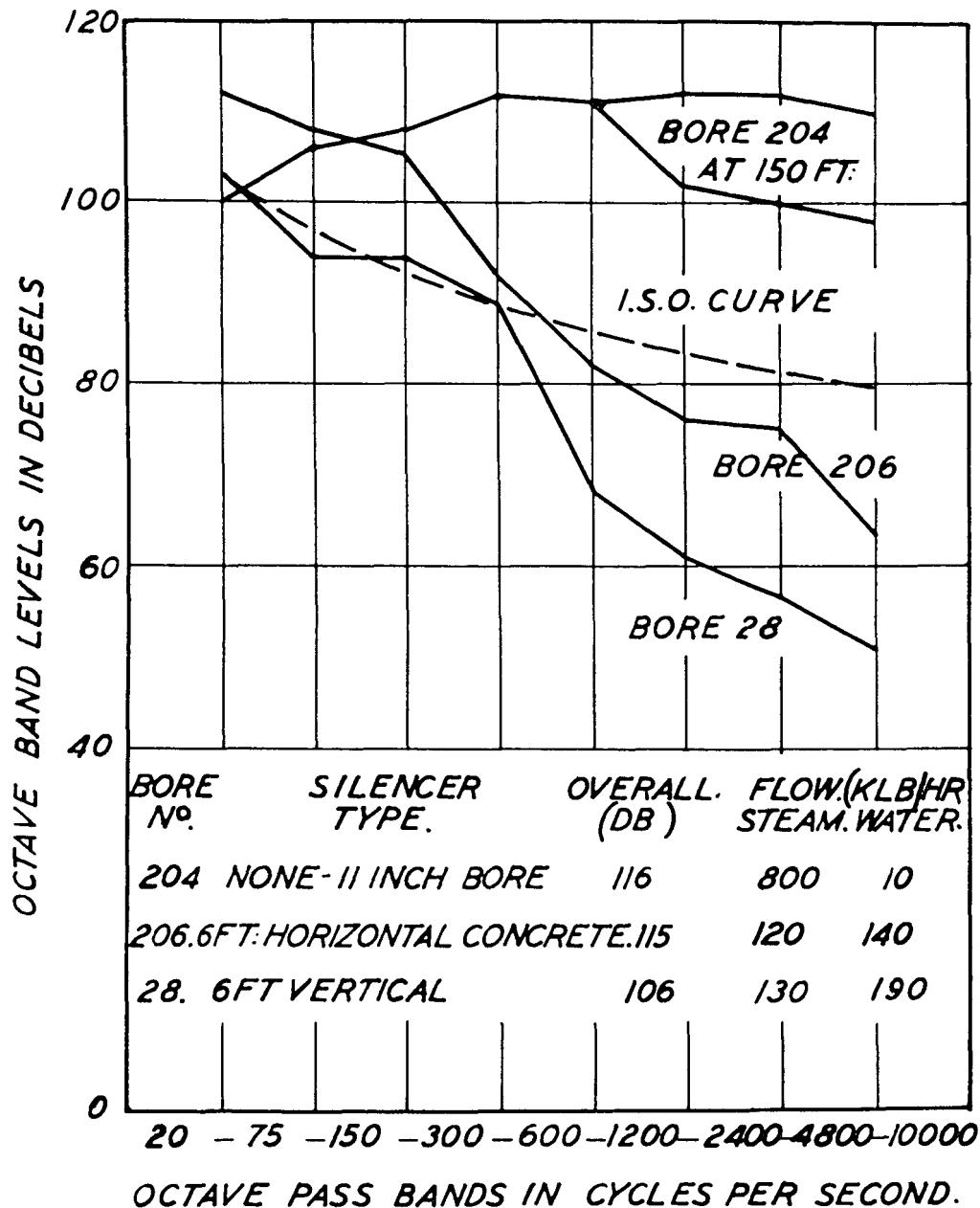
Figure 3. Sound levels at 42 feet (13 m)
