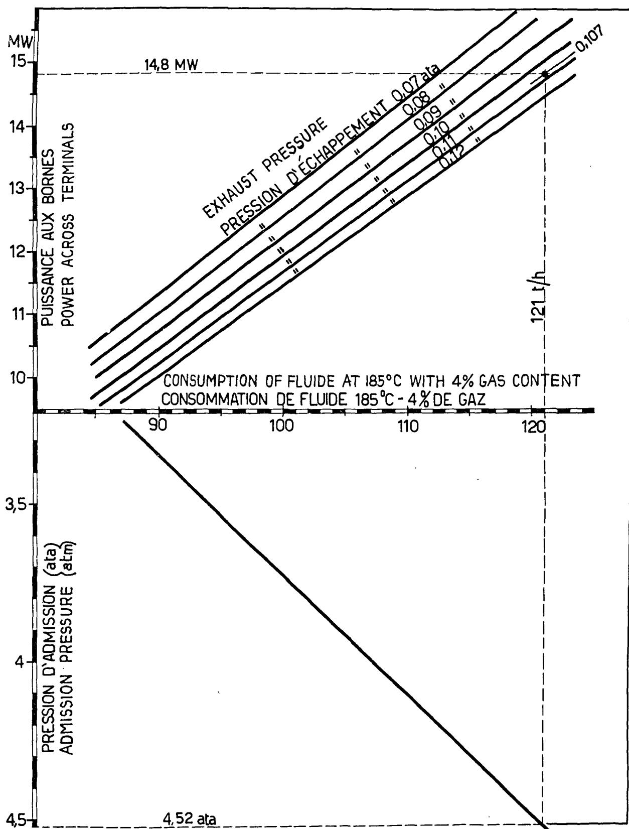
Figure 8. Consumption curves of 1 500 kW unit
