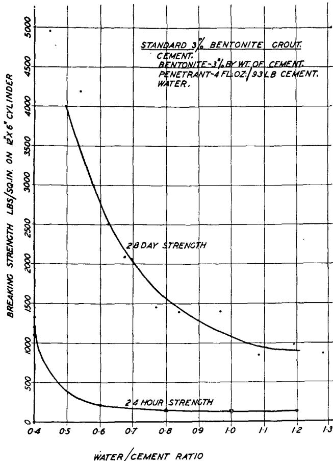
Figure 6. 24-hour and 28-day strengths of N.Z. cement normal slurries
