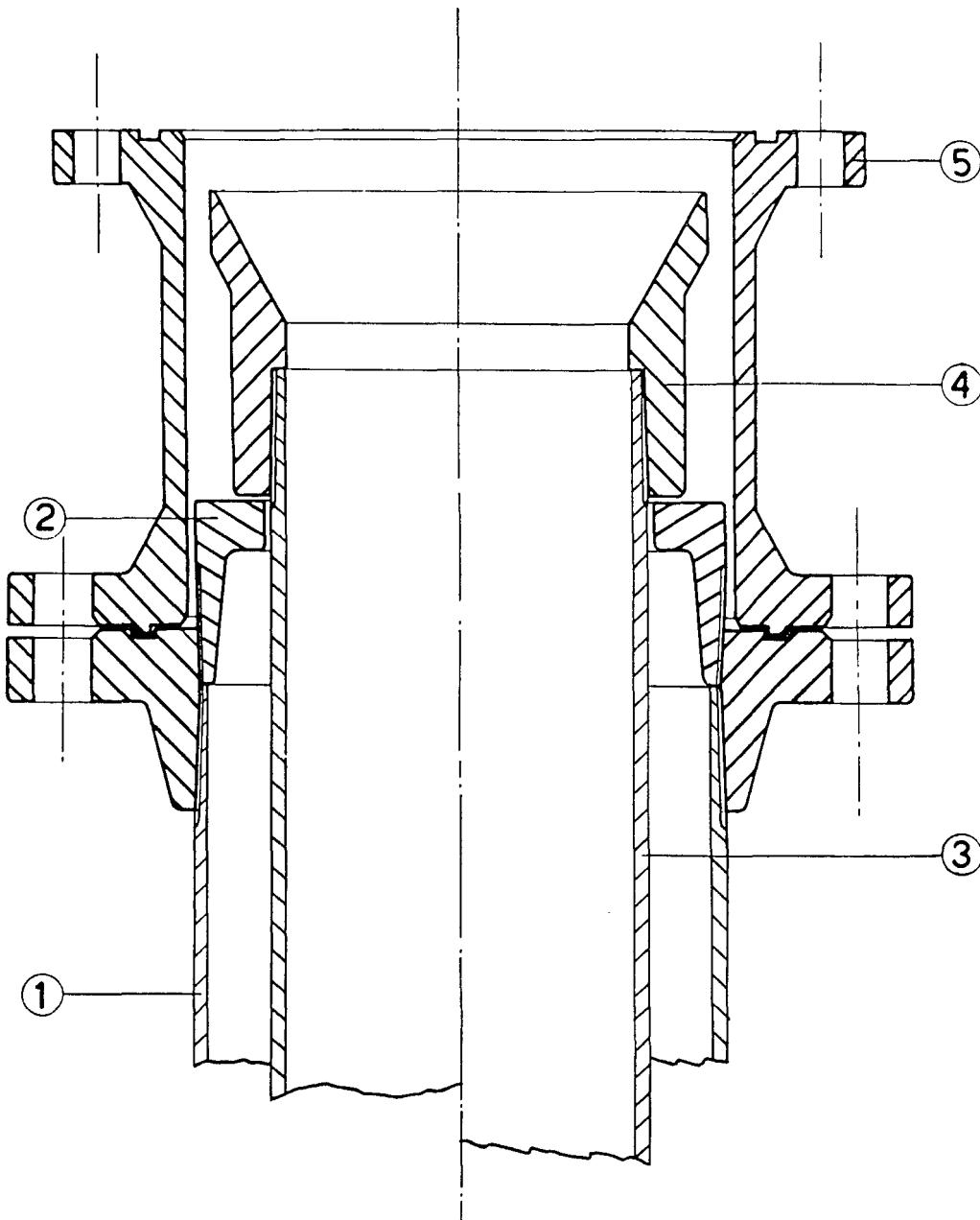
Figure 1. Casing head in a natural-steam production well
