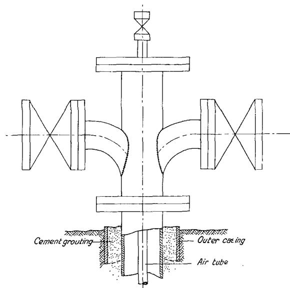
Figure 1. Diagrammatic representation of standard well-head
