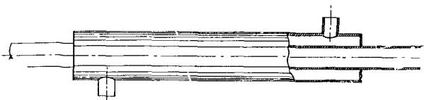
Figure 2. Simple tube and jacket exchanger
