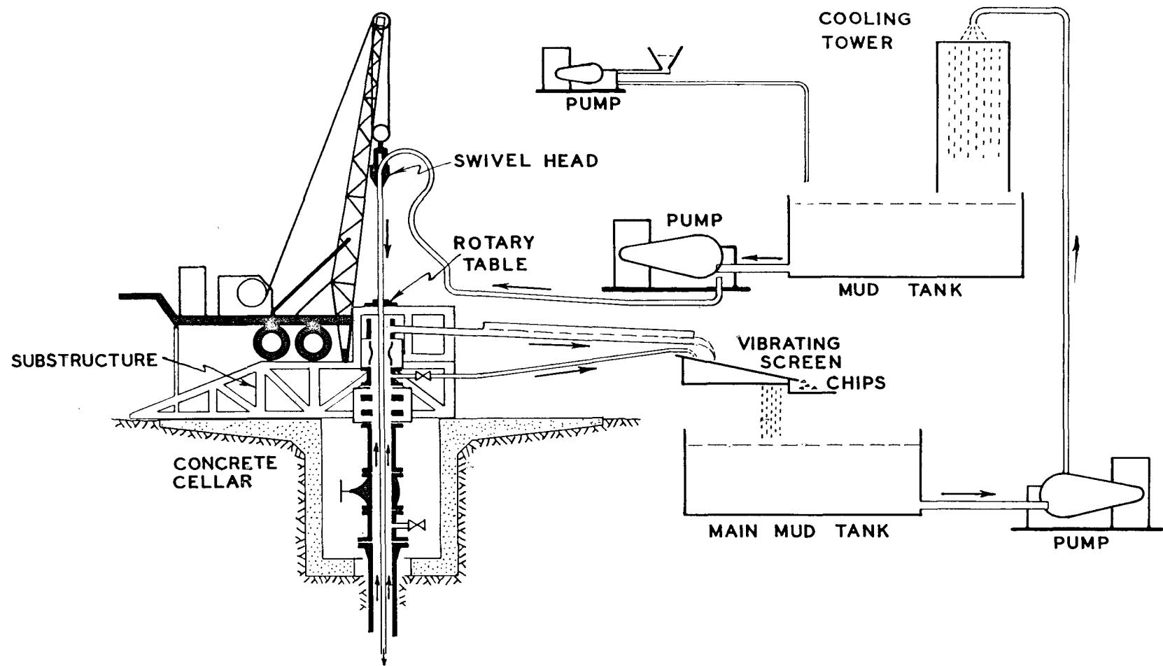
Figure 2. Typical rig and circulation layout
