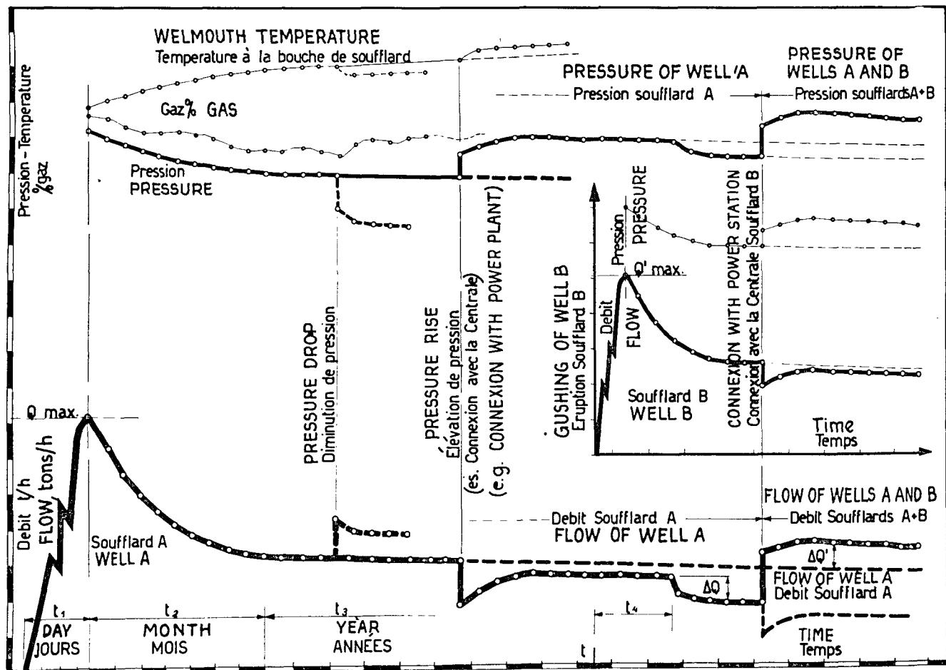
Figure 13. Operation of steam wells without shutdown equipment
