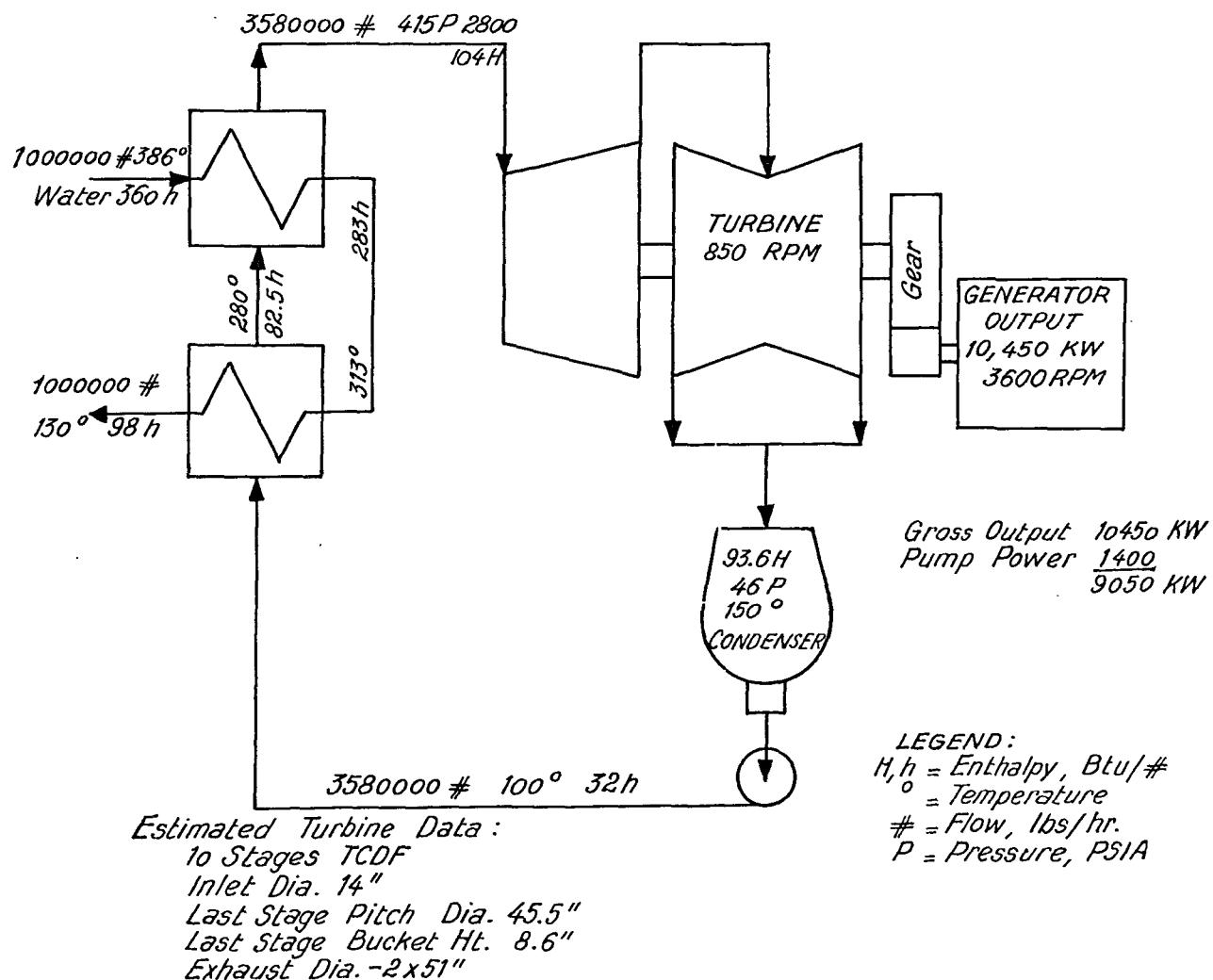
Figure 7. Freon cycle (F-114) for geothermal application
