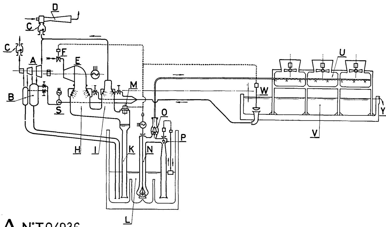
Figure 7. General scheme with underlying condenser
