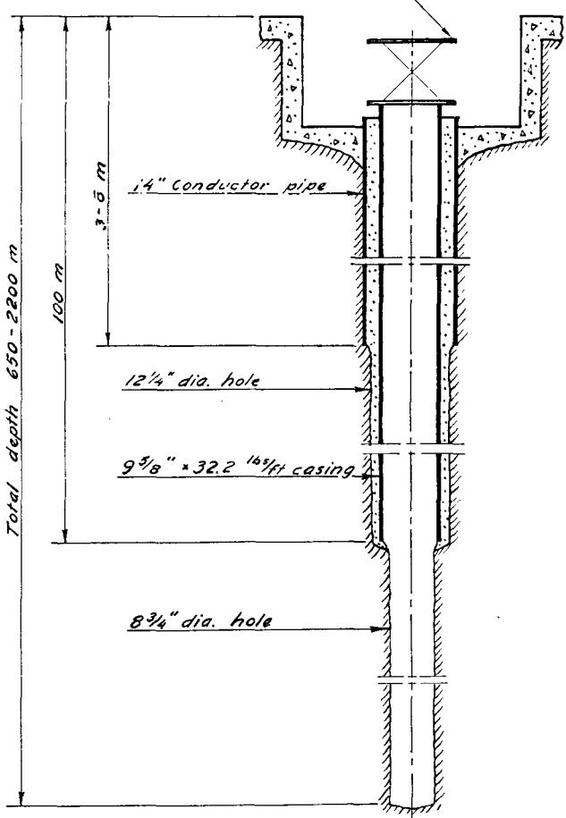
Figure 5. Drilling and casing programme
