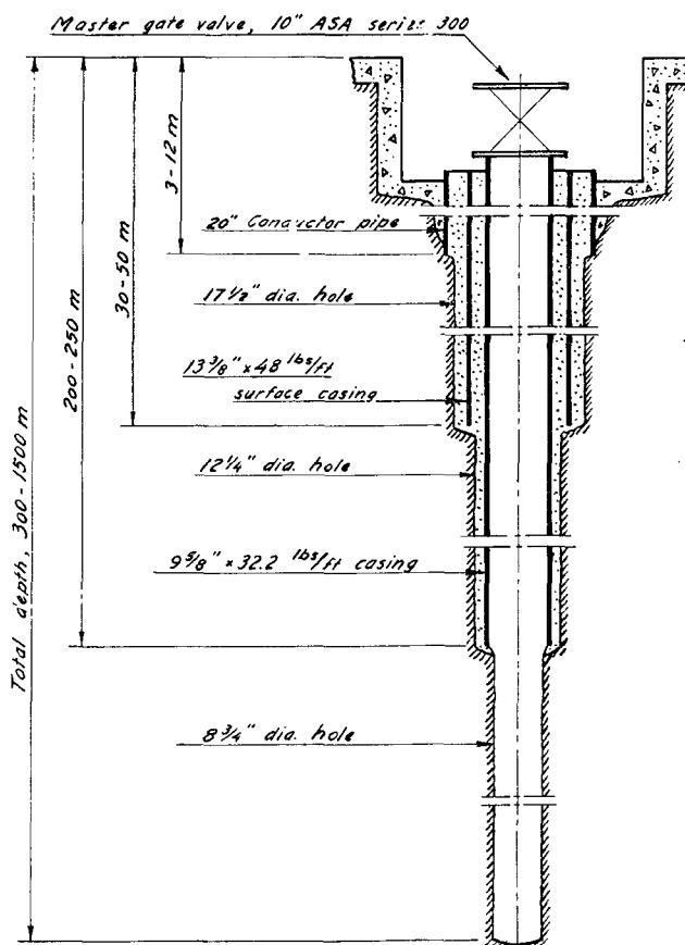
Figure 4. Drilling and casing programme
