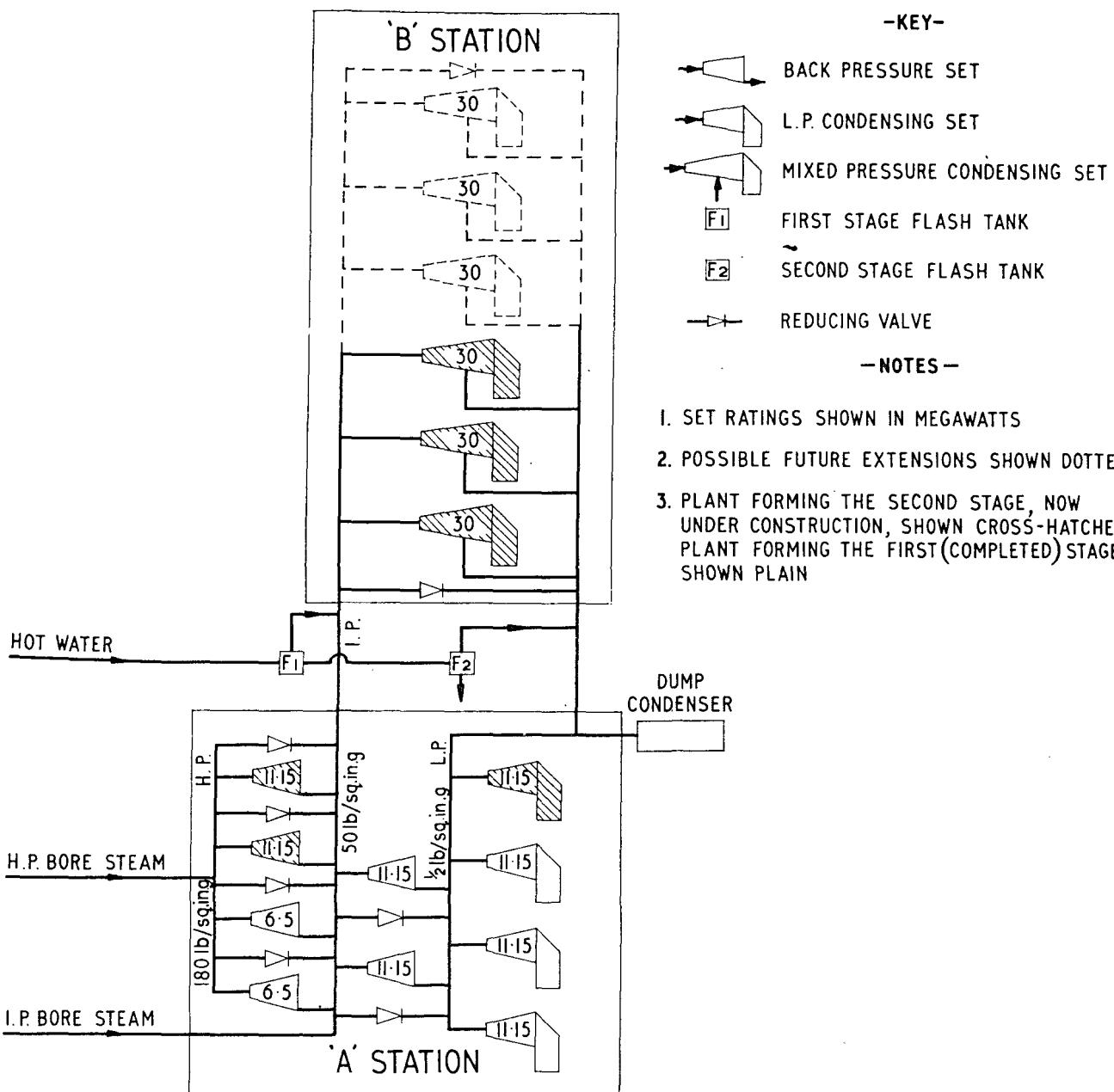
Figure 2. Arrangement of generating plant
