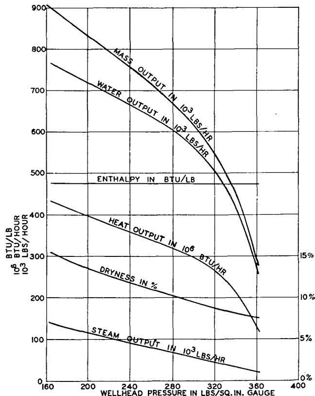
Figure 3. Output curves for bore 81
