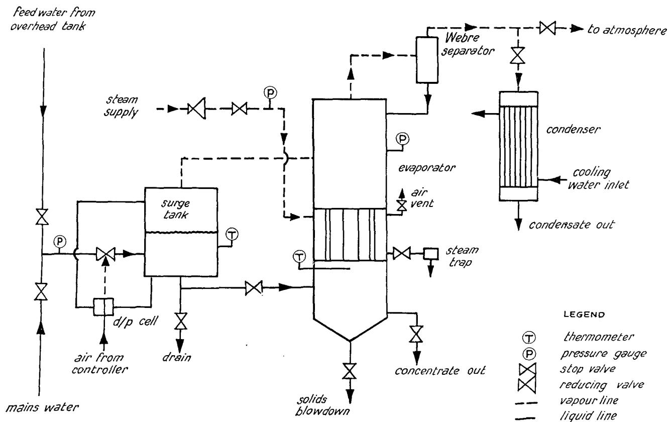
Figure 7. Sketch of evaporator layout
