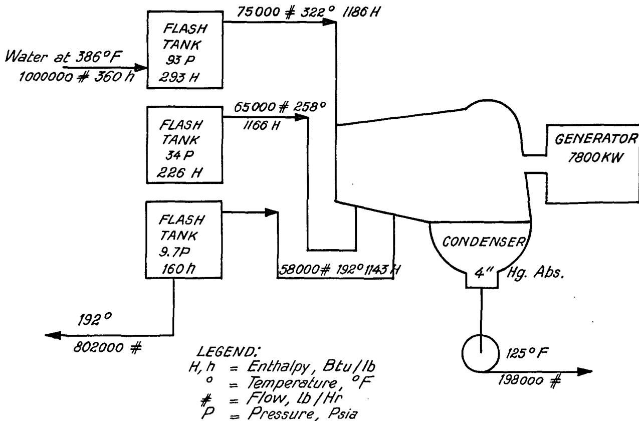
Figure 3. Multiple flashing cycle for geothermal application
