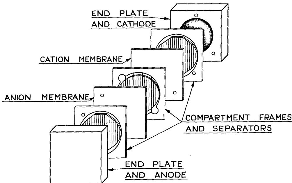
Figure 1. Exploded view of cell assembly
