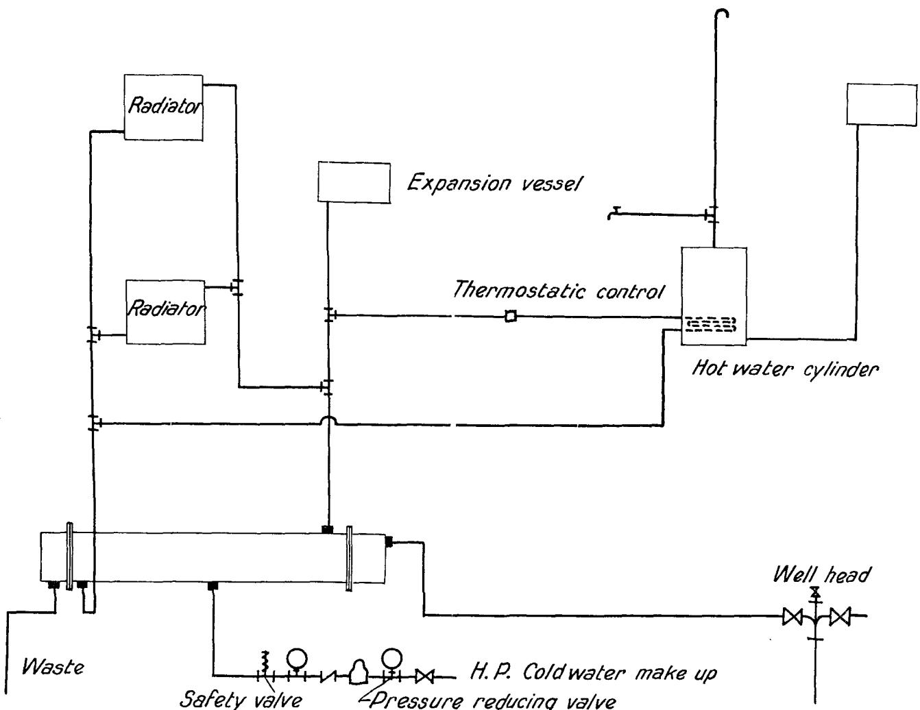
Figure 4. Line diagram of closed system
