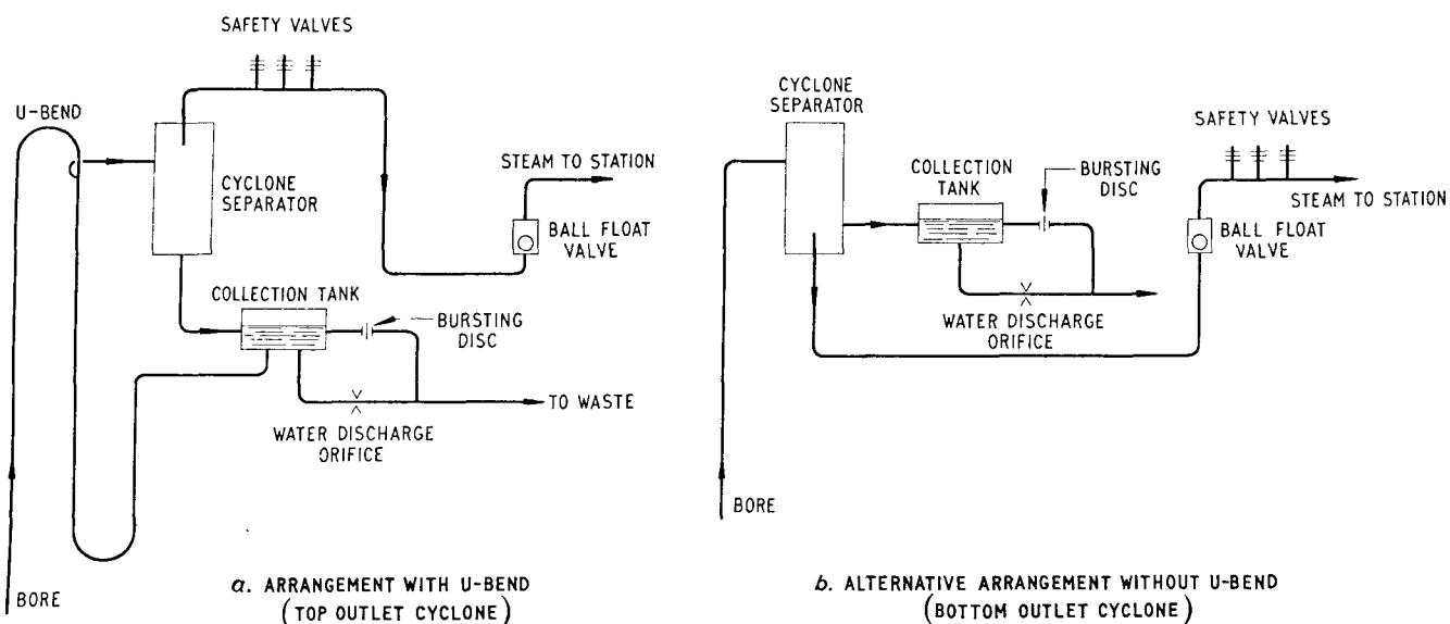
Figure 3. Diagram of wellhead equipment
