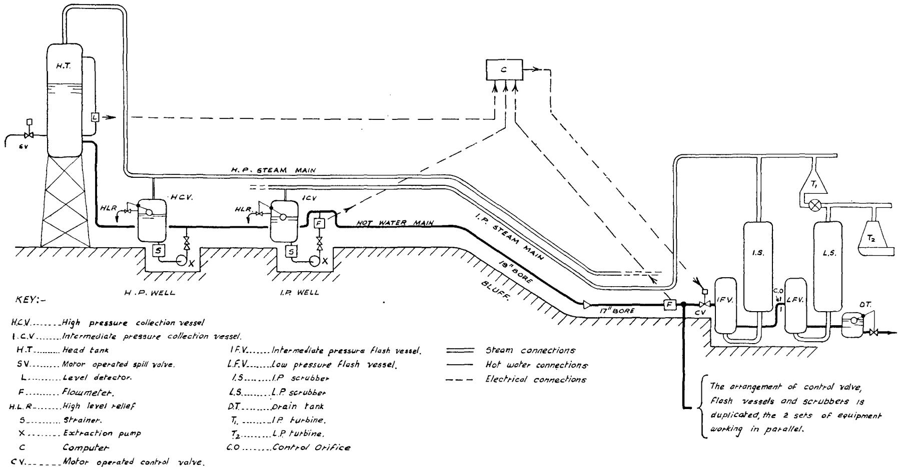
Figure 4. Diagram of hot water transmission system
