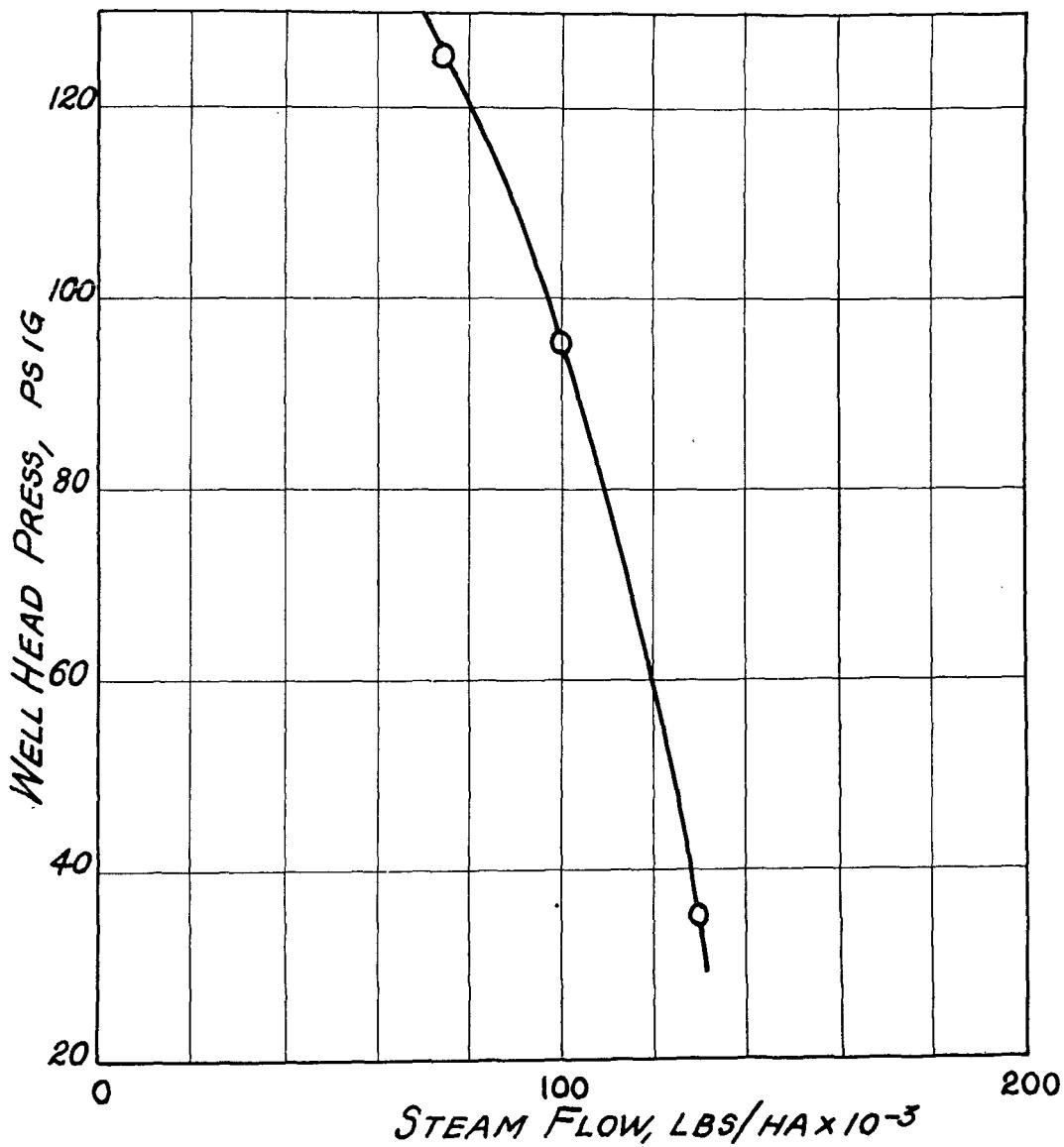
Figure 5. Magma No. 1 full flow test, 16 Nov. 1960
