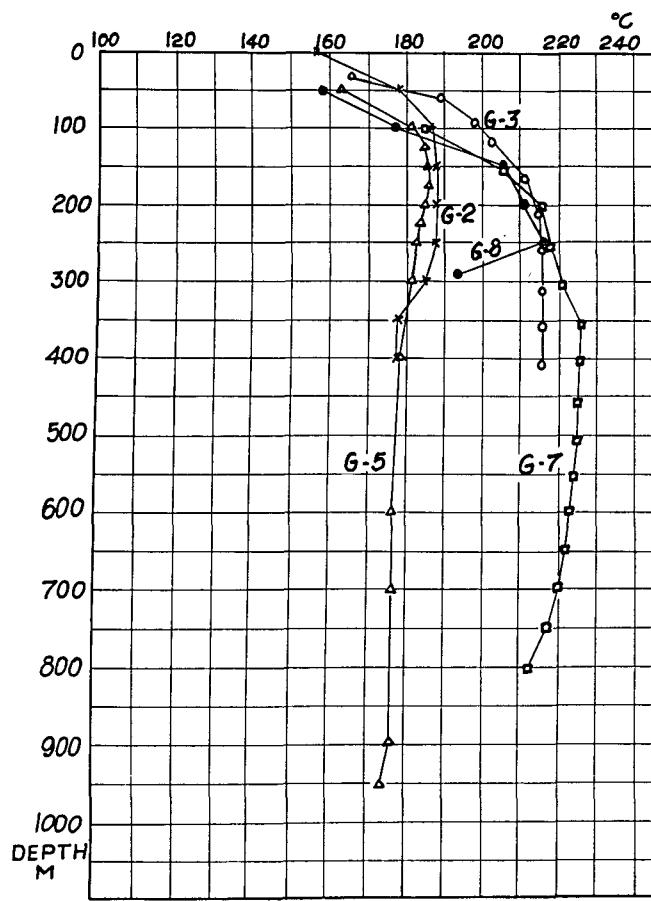
Figure 5. Measured temperatures in steam wells at Hveragerði
