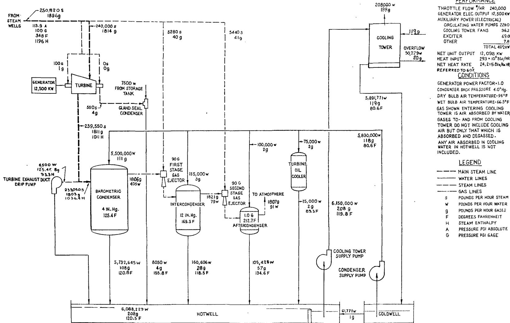
Figure 3. The Geysers power plant: heat balance diagram, unit No. 1
