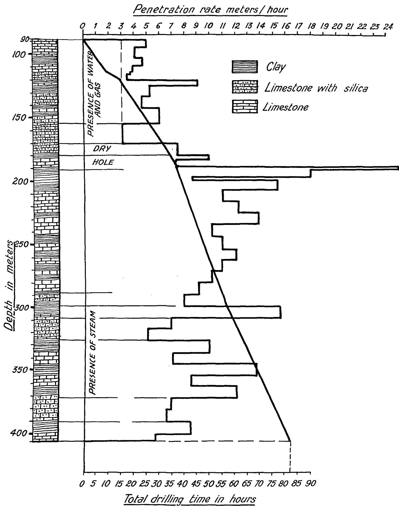
Figure 2. Air drilled exploratory hole (drilling time/penetration rate)
