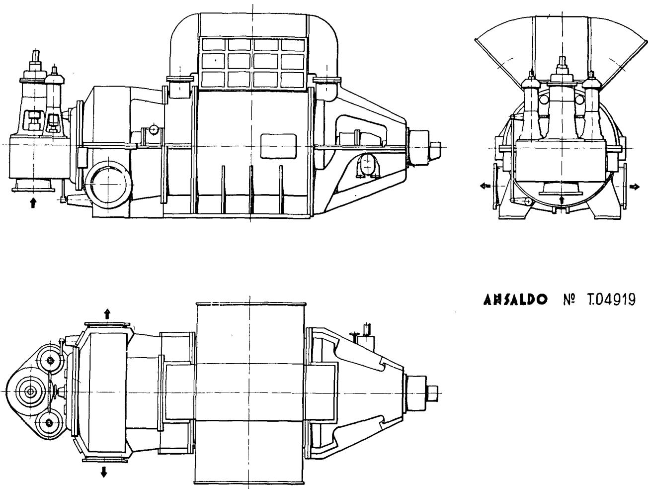
Figure 2. 3 000-3 500 kW turbine-generator set
