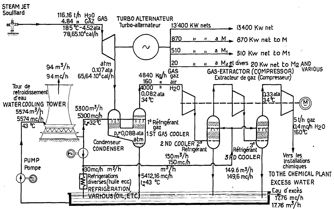
Figure 3. Natural steam condensing power plant (scheme 3)
