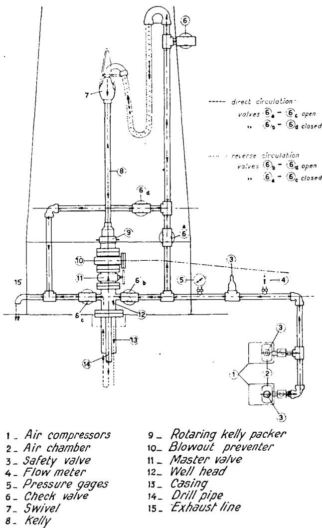
Figure 1. Surface equipment and stand-pipe arrangement for air drilling with direct and reverse circulation
