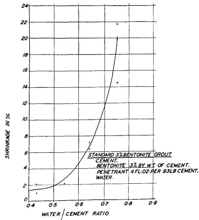
Figure 2. Shrinkage v. water/cement ratio for normal N.Z. cement slurries
