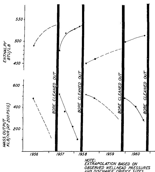
Figure 2. Changes in mass and enthalpy resulting from mineral deposition in a bore
