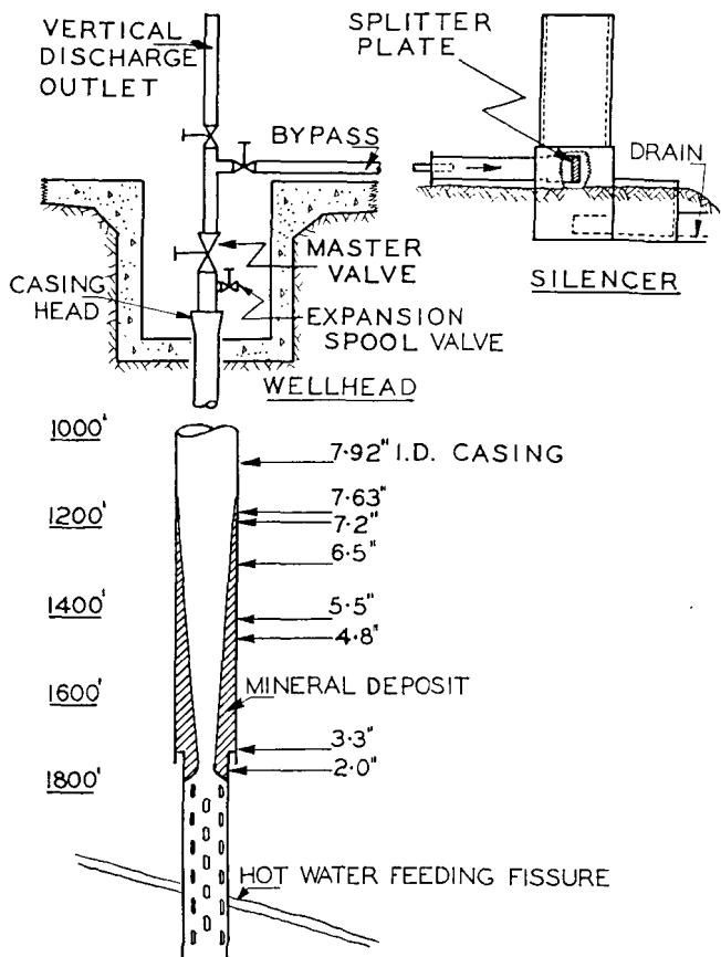
Figure 3. Typical mineral deposit build-up in a bore casing
