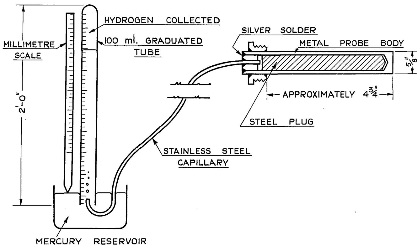
Figure 3. Hydrogen probe
