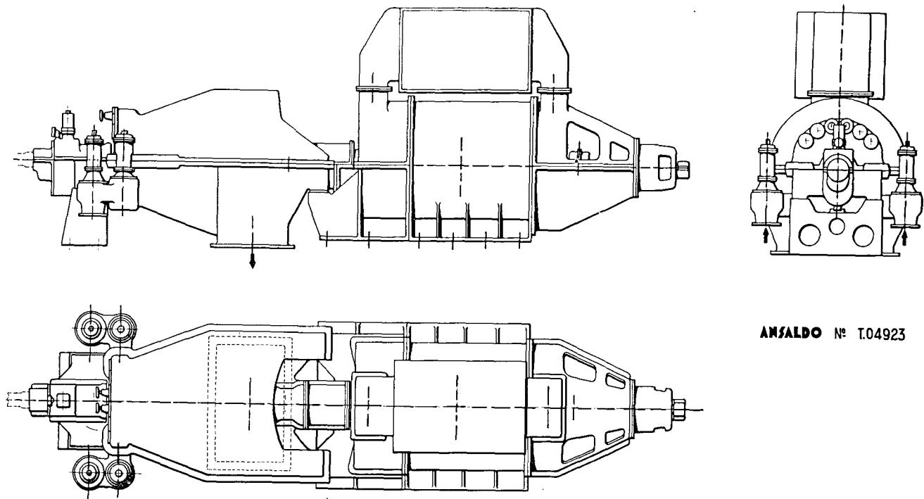
Figure 4. 7 000 kW turbine-generator set
