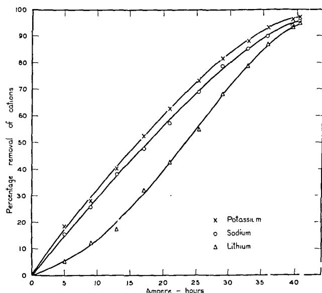
Figure 4. Selective removal of cations in batchwise desalting of bore water
