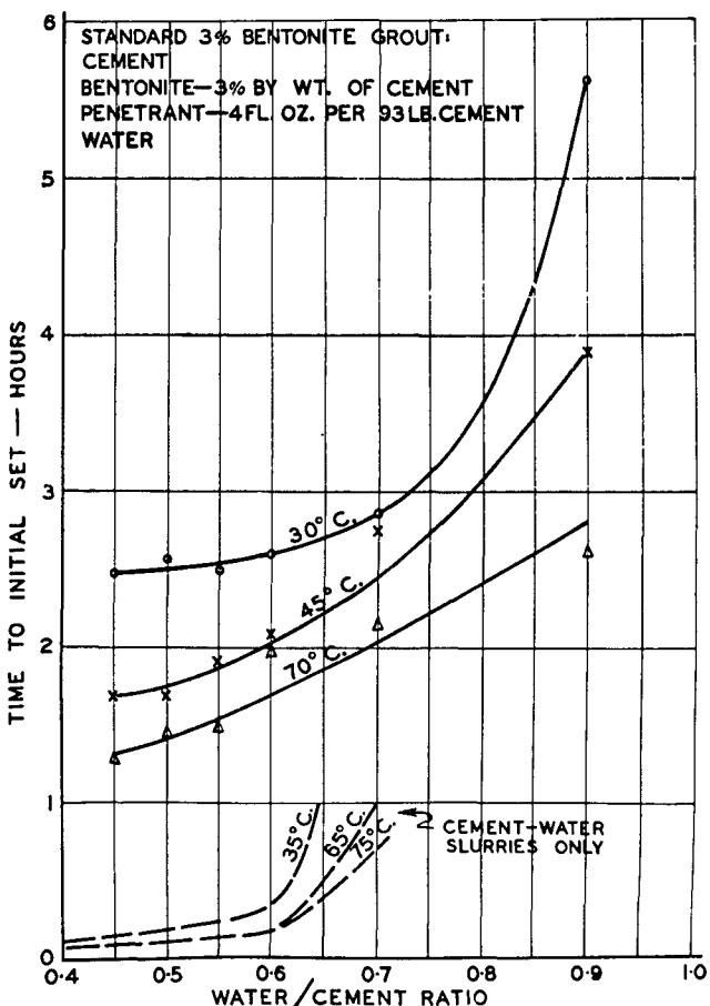
Figure 3. Setting times v. water/cement ratio for normal N.Z. cement slurries
