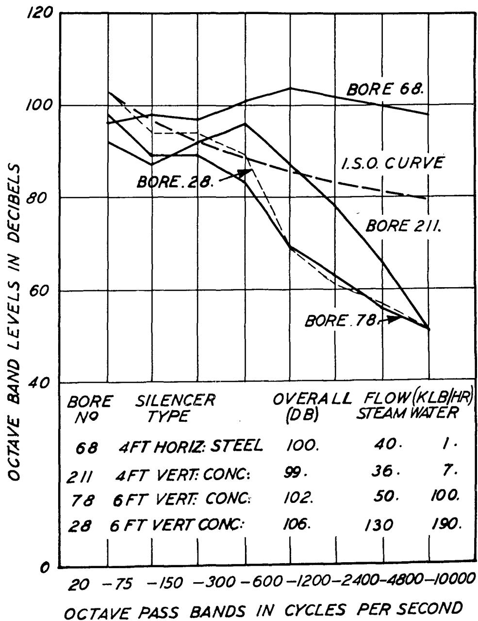
Figure 4. Sound levels at 2 feet (13 m)
