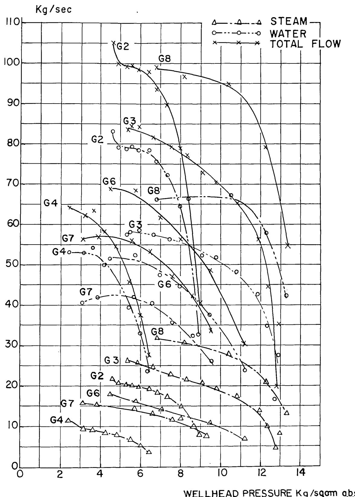
Figure 2. Flow characteristics of steam wells at Hveragerði. The yield is measured at zero gauge (100°C)
