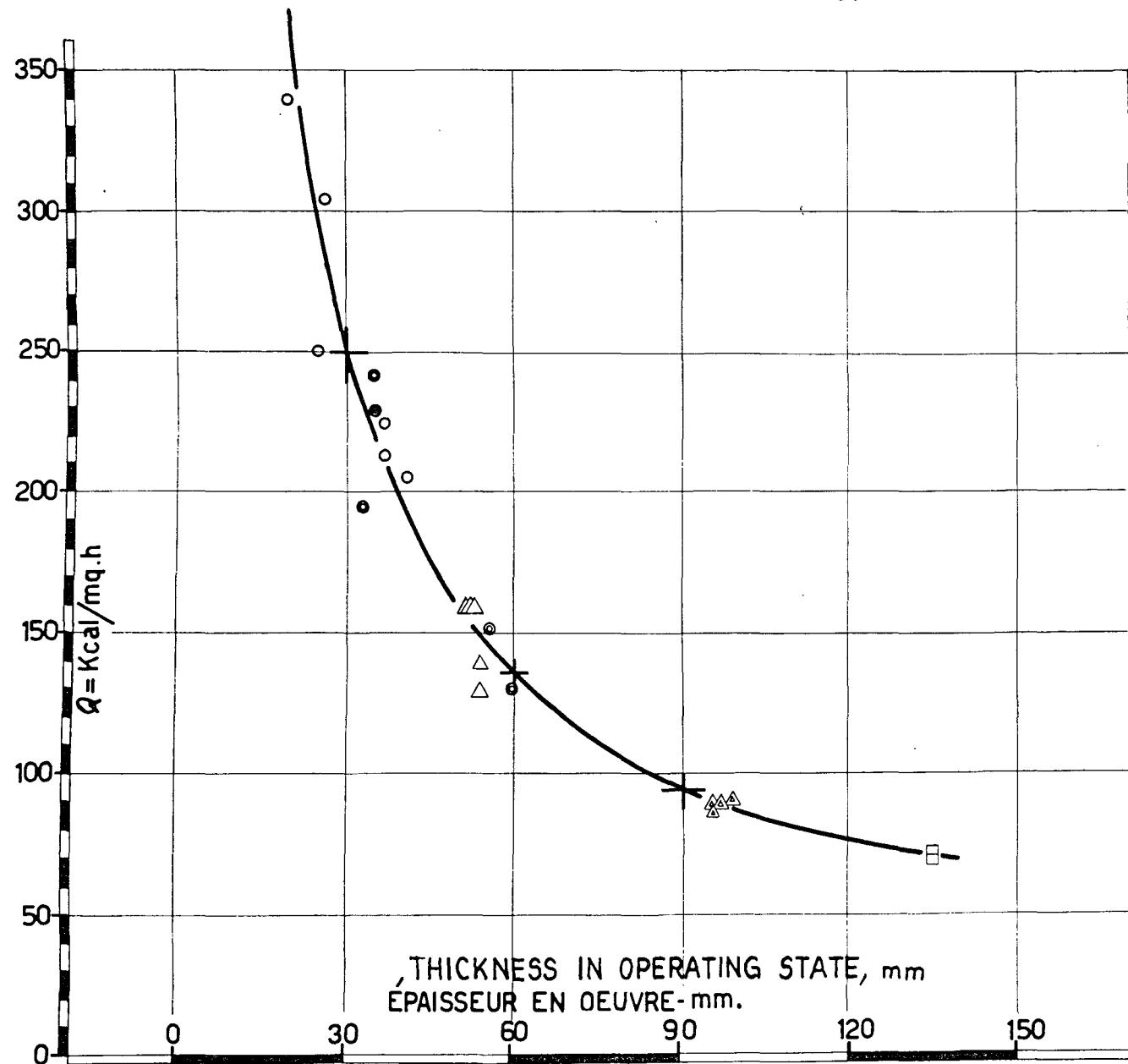
Figure 15. Over-all heat-transfer coefficient for thermal insulating materials
