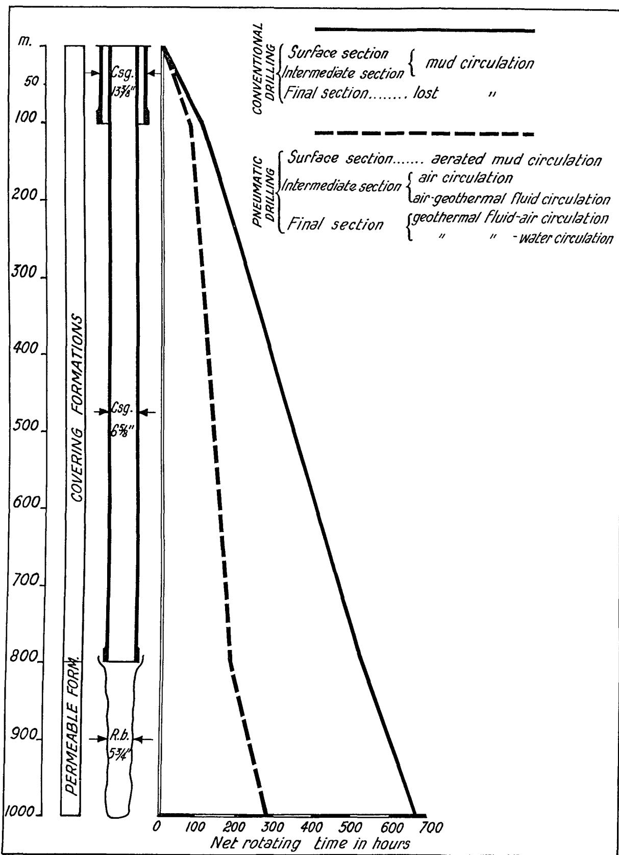
Figure 5. Comparison between conventional and pneumatic drilling time for an exploratory geothermal bore
