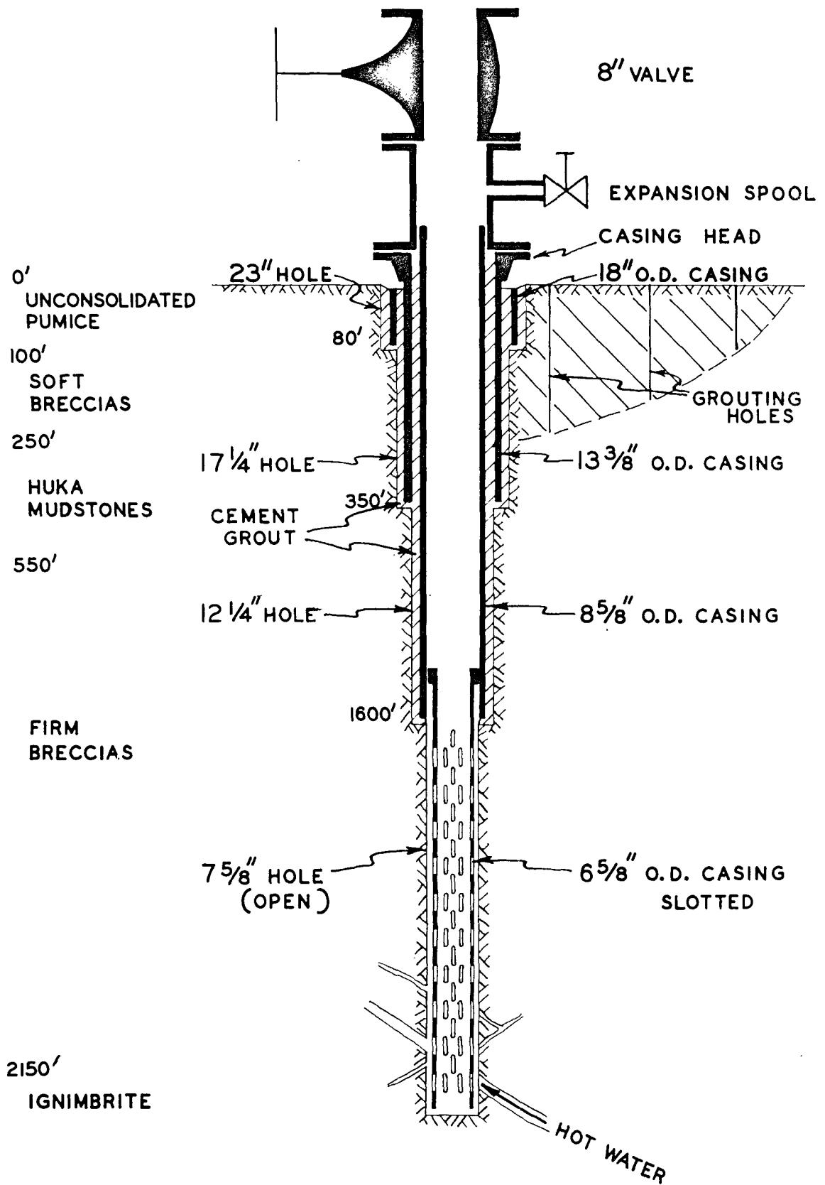
Figure 1. Casing layout and geological formations
