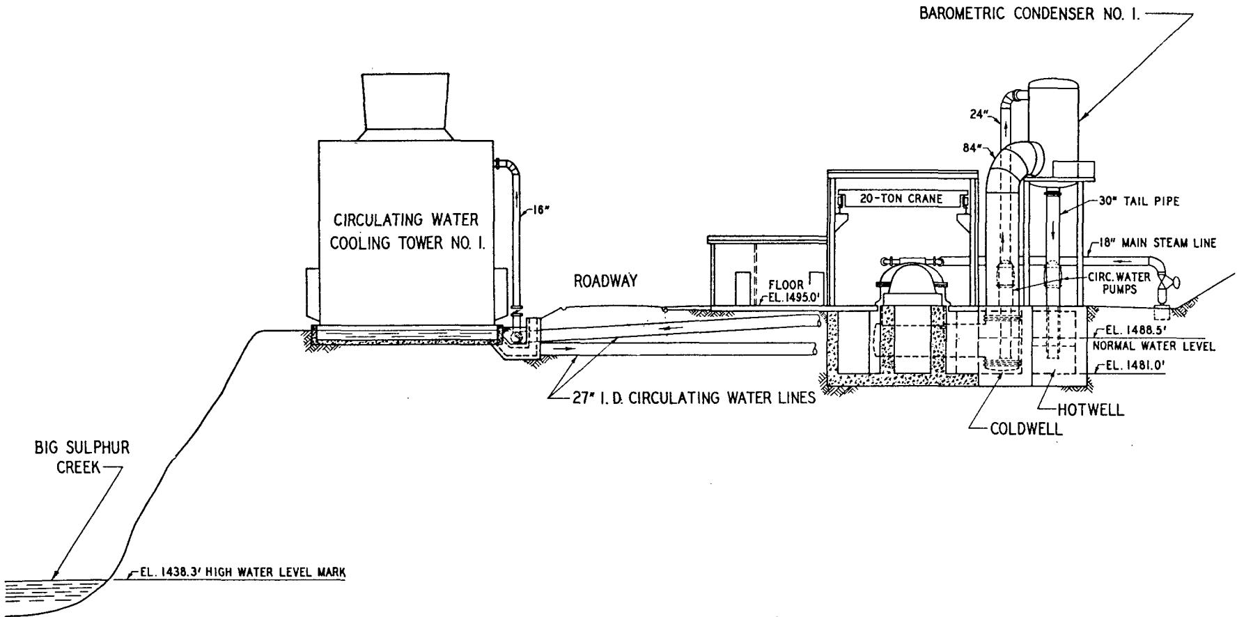
Figure 5. The Geysers power plant: elevation
