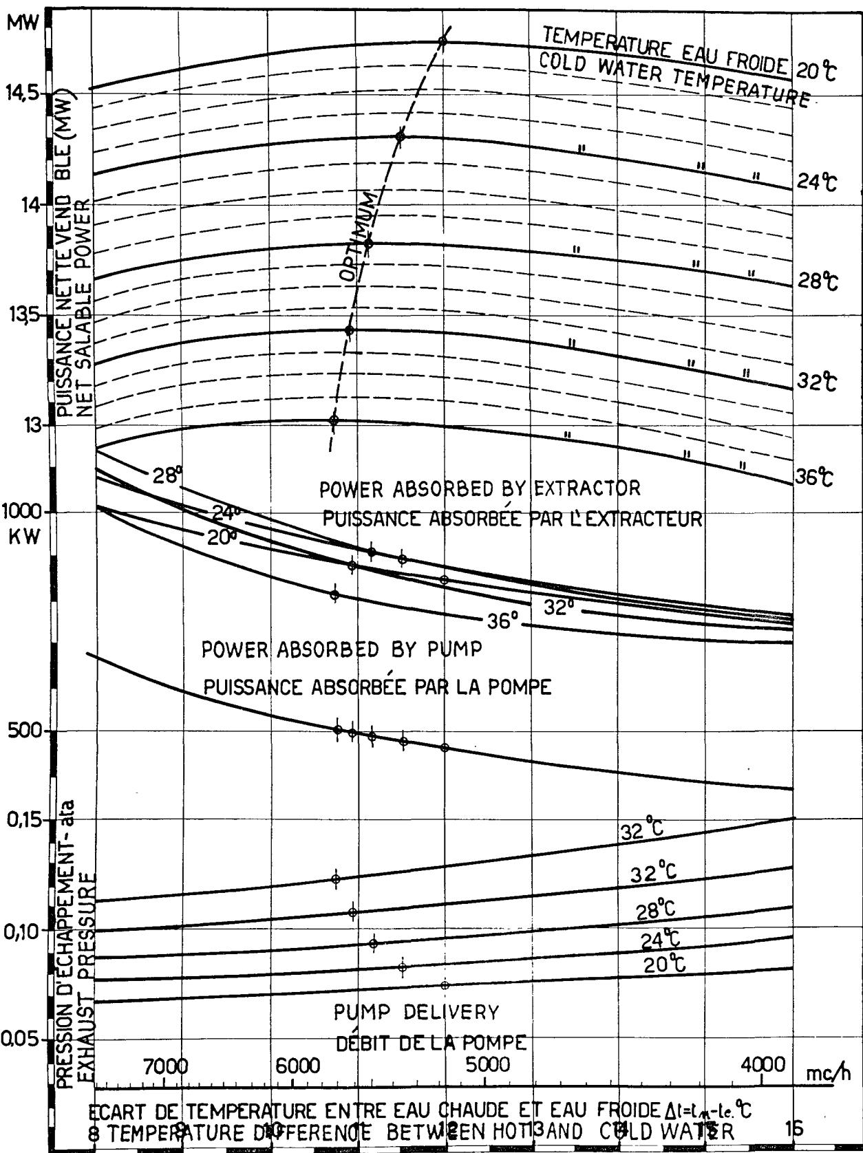
Figure 11. Finding the optimum for the auxiliaries of a natural steam unit
