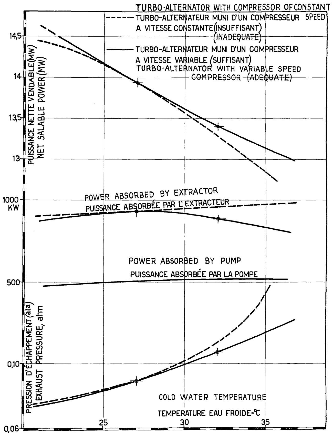
Figure 12. Operation of condenser turbo-alternators on natural steam
