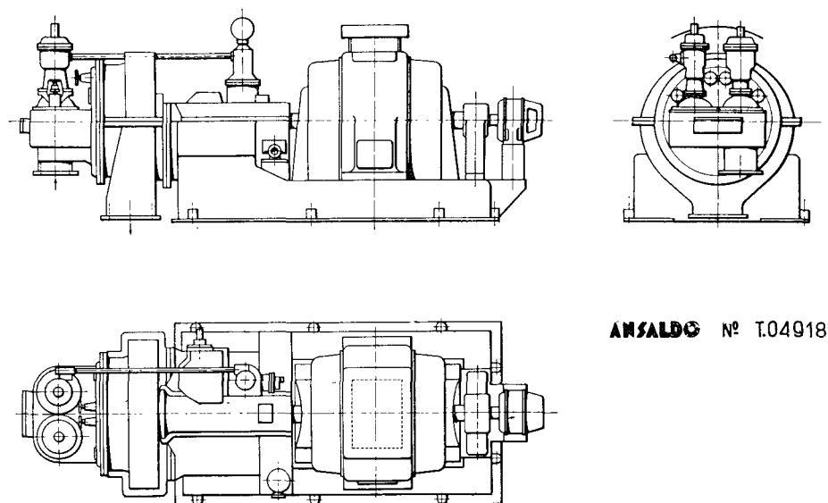
Figure 1. 900-1 250 kW turbine-generator set
