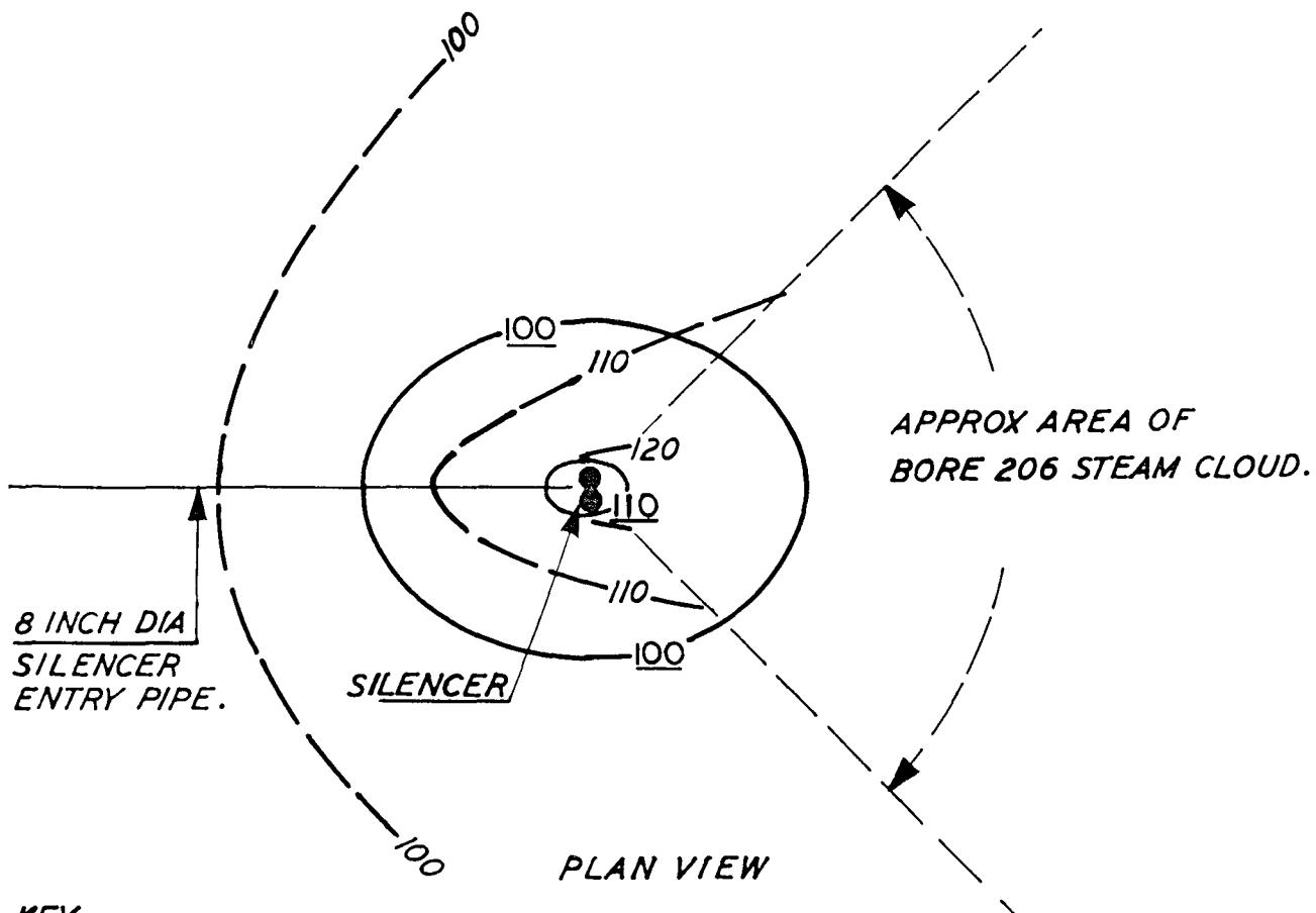
Figure 5. Over-all sound level contours
