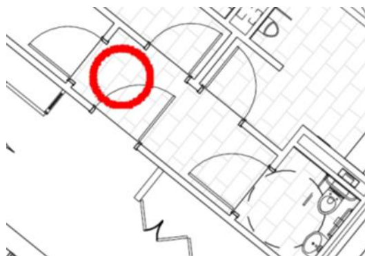
Figure IX Corridor with insufficient manoeuvring space
