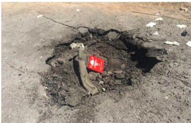
Crater configuration is not typical of explosion of aerial chemical munition
