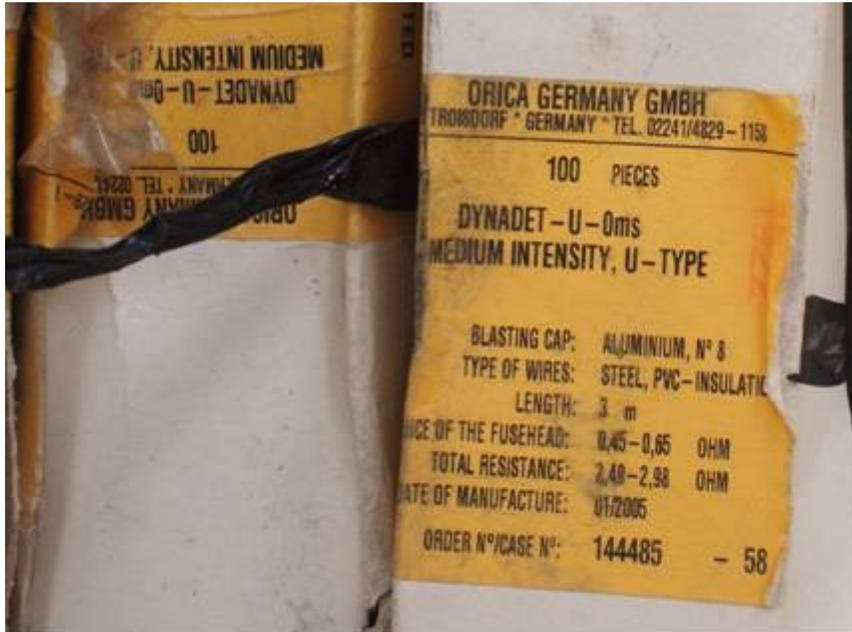
*Electric detonators, manufactured in Germany, Garowe, 11 November 2012*
