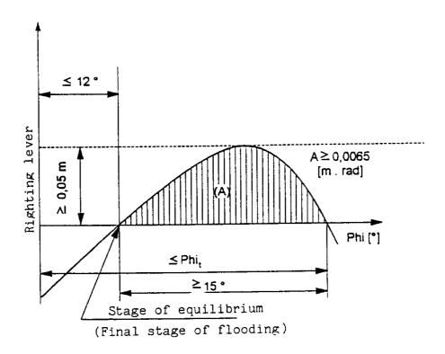
(3) Inland navigation vessels carrying containers which have not been secured shall satisfy the following damage stability criteria:
