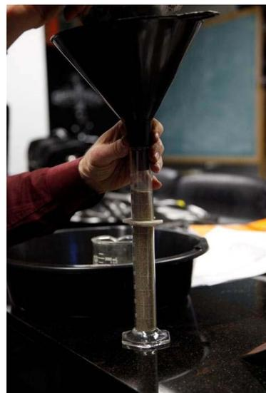
4. Common beach sand was for the indentation volume displacement measurements with the following particle size analysis: 78.0% Thru 250 micron screen, 16.6% Thru 149 micron screen, 3.9% Thru 105 micron screen, 1.0% Thru 74 micron screen, 0.2% Thru 53 micron screen, 0.06% Thru 44 micron screen and 0.14% Residue On 37 micron screen.
