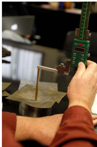
3. In addition, each set of three 1.219 mm and 0.912 mm steel witness plates for those same 19 compositions which did not puncture through were measured for average and maximum displacement volumes in milliliters of dry fine sand (see Figures 3 through 5 below for technique of measurement.) For each set of three trials, the average and maximum (of 3) indentation volume data for both the 1.219 mm and 0.912 mm witness plates is summarized in columns 5, 6, 9 and 10 of Table IA below
