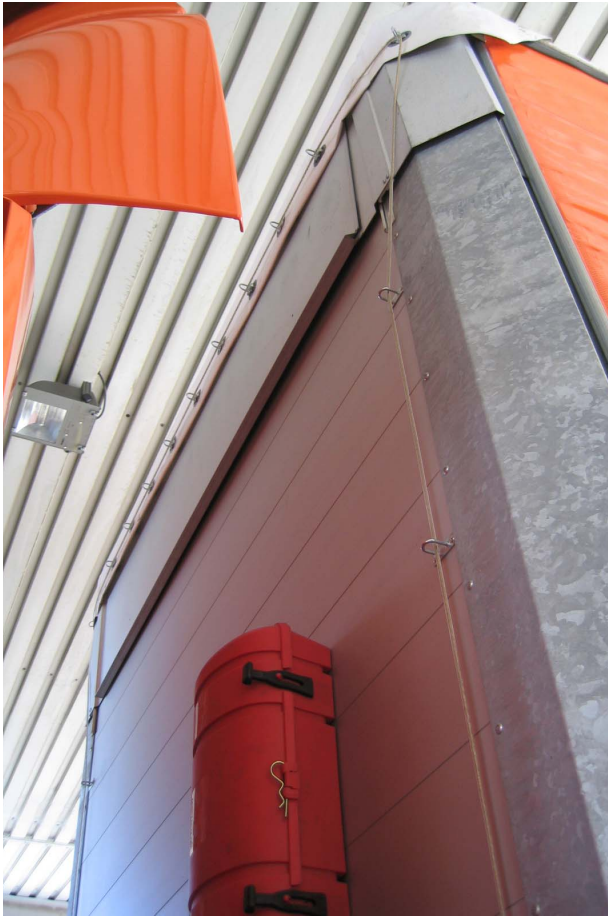
A: Metal TIR rings mounted onto the solid part of the trailer and reinforced eyelets at the edge of the sheet. The upper part of the sheet is then secured and kept in place by the TIR wire. This system requires a rather long TIR wire – approximately 7 meters extra compared to a standard TIR wire.
