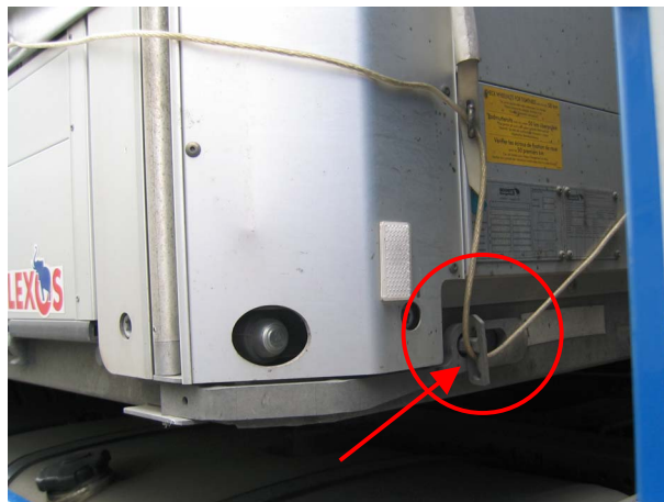
Lock tab secured by the TIR wire.
