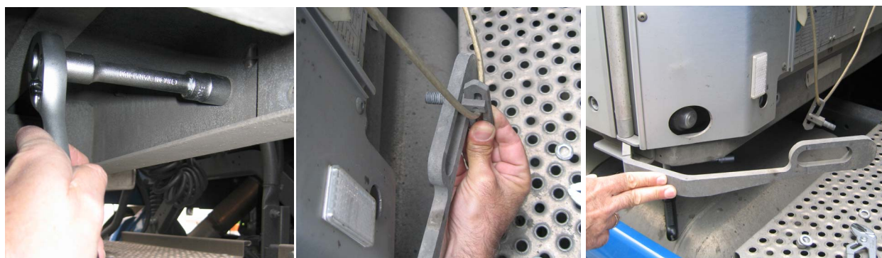
Inner side of the chassis frame – the lock tab nut is NOT secured.
