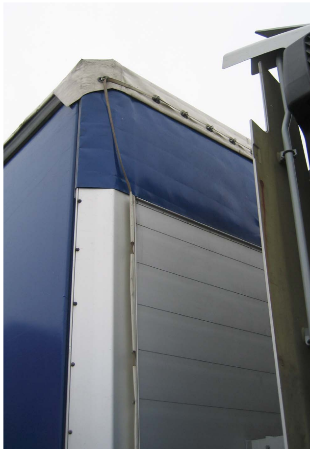
B: Metal TIR rings mounted onto the solid part of the trailer and reinforced eyelets at the edge of the sheet. The upper part of the sheet is then secured and kept in place by a thong made of material and in dimensions as prescribed by the TIR Convention. The TIR wire will secure the lower part of the thong. Normal length TIR wire required for this system.
