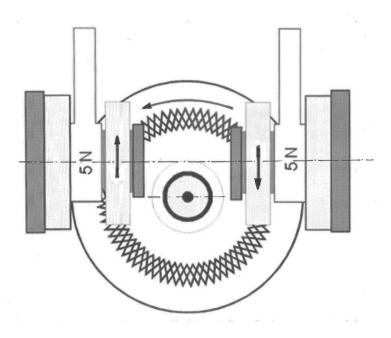
Two weighted parallel arms each carrying a special abrasive wheel freely rotating on a ball-bearing horizontal spindle; each wheel rests on the test specimen under the pressure exerted by a mass of 500 g.
