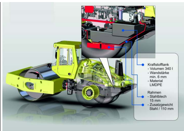
Inherently safe design of the fuel tank in a single drum compactor
