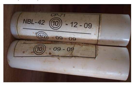
Label of a transportation container for propellant charges CP-1, Lot No. 10-29-09, manufactured in Bulgaria in 2009, and used in the production of 40mm rounds RF-7MA, Bosaso, 7 December 2012
