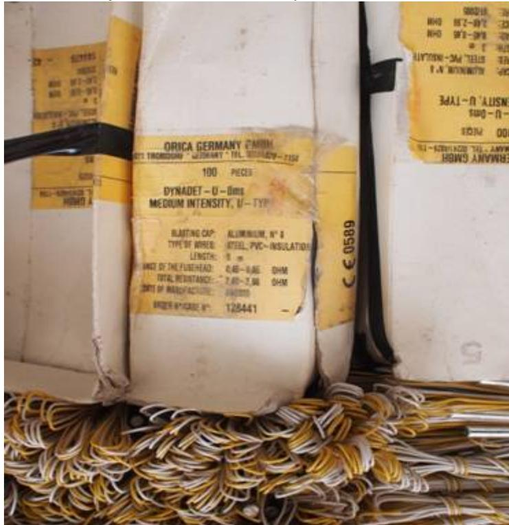
*Electric detonators, manufactured in Germany in 2004, Garowe, 11 November 2012*
