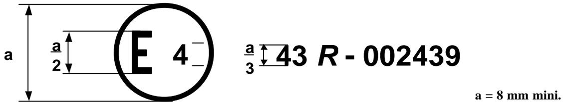
The above approval mark affixed to a vehicle shows that the vehicle type concerned has, with regard to installation of glazing, been approved in the Netherlands (E 4) pursuant to Regulation No. 43. The approval number indicates that the approval was granted in accordance with the requirements of Regulation No. 43.
