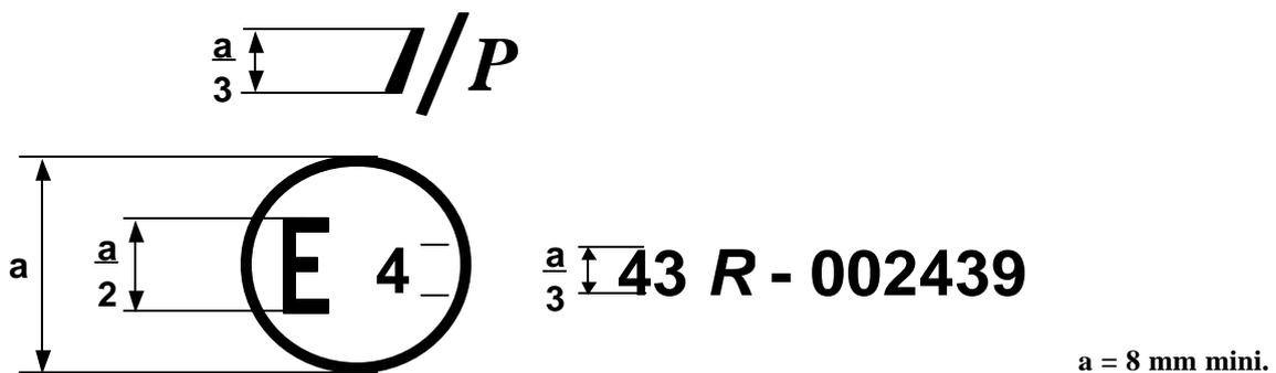
The above approval mark affixed to a toughened-glass windscreen faced with plastics material shows that the component concerned has been approved in the Netherlands (E 4) pursuant to Regulation No. 43 under approval No. 002439. The approval number indicates that the approval was granted in accordance with the requirements of Regulation No. 43.
