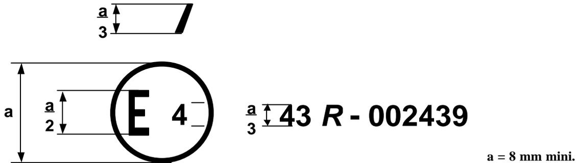
The above approval mark affixed to a toughened-glass windscreen shows that the component concerned has been approved in the Netherlands (E 4) pursuant to Regulation No. 43 under approval number 002439. The approval number indicates that the approval was granted in accordance with the requirements of Regulation No. 43.
