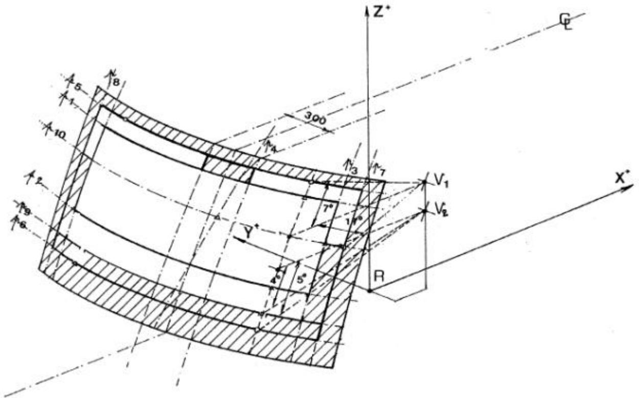
$C_L$  : trace of the longitudinal median plane of the vehicle
