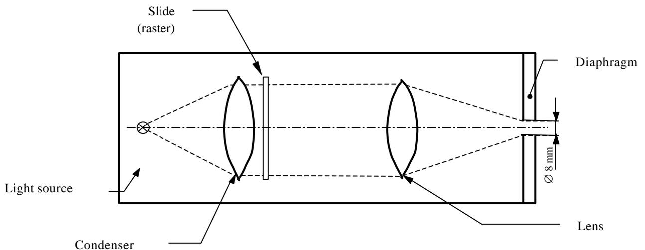
Figure 7: Optical arrangement of the projector
