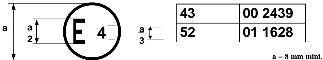
The above approval mark affixed to a vehicle shows that the vehicle type concerned has been approved in the Netherlands (E 4) pursuant to Regulations Nos. 43 and 52 <sup>3/</sup>. The approval numbers indicate that, at the date when the respective approvals were given, Regulation No. 43 was in its original form and Regulation No. 52 included the 01 series of amendments.
