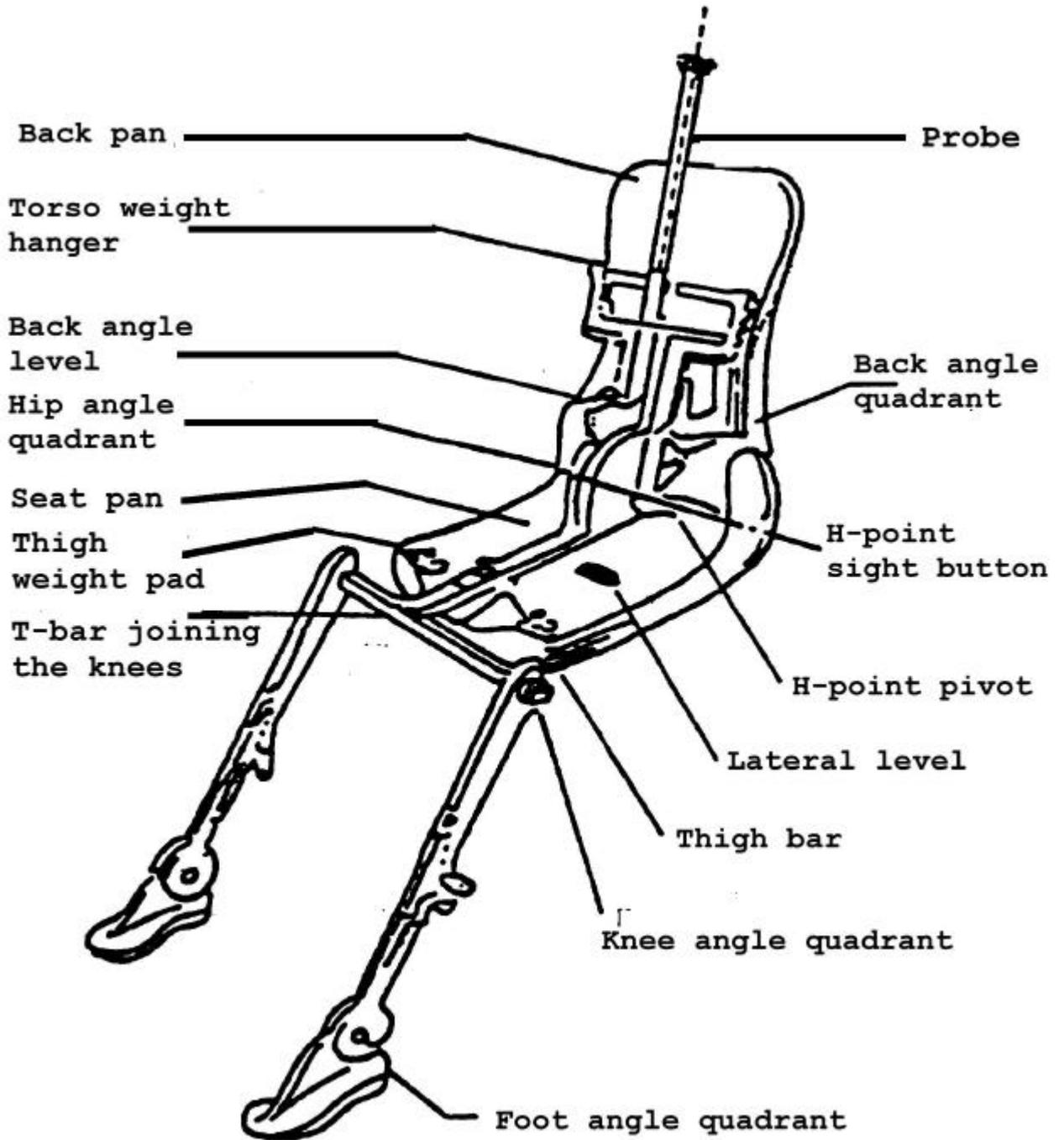
Figure 1: Designation of 3 DH machine components
