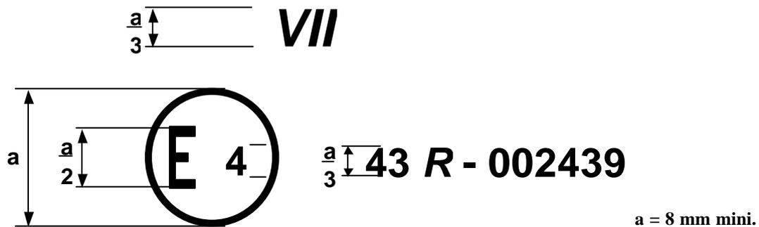
The above approval mark affixed to a uniformly-toughened glass pane shows that the component concerned intended to be used as a windscreen on a slow-moving vehicle which, by construction, cannot exceed 40 km/h, has been approved in the Netherlands (E 4) pursuant to Regulation No. 43 under approval No. 002439. The approval number indicates that the approval was granted in accordance with the requirements of Regulation No. 43.
