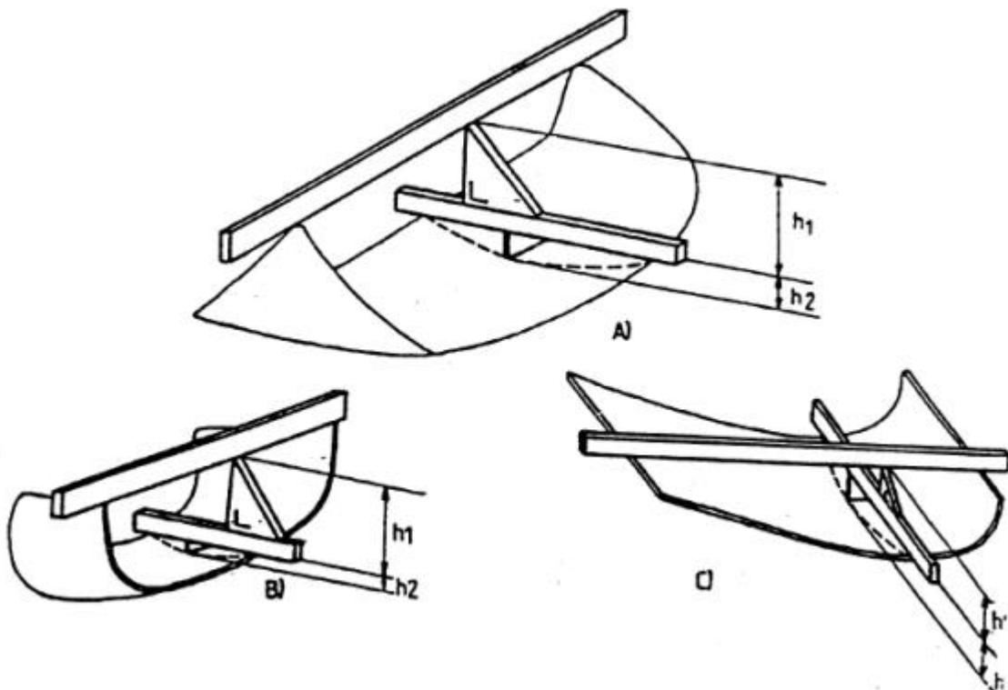
Figure 1: Determination of the height of segment 'h'
