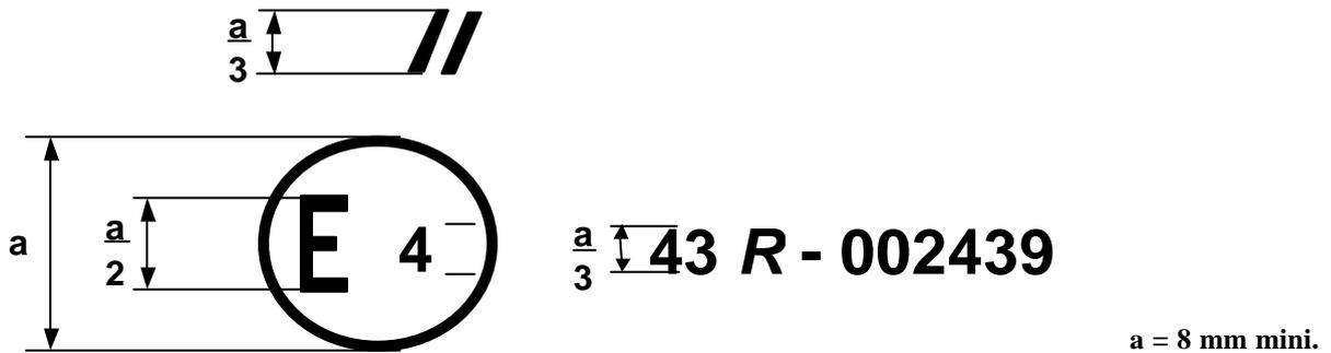
The above approval mark affixed to an ordinary laminated-glass windscreen shows that the component concerned has been approved in the Netherlands (E 4) pursuant to Regulation No. 43 under approval No. 002439. The approval number indicates that the approval was granted in accordance with the requirements of Regulation No. 43.
