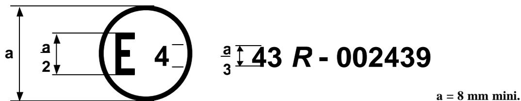
The above approval mark affixed to a glass pane other than a windscreen to which the requirements of annex 3, paragraph 9.1.4.1., are applicable shows that the component concerned has been approved in the Netherlands (E 4) pursuant to Regulation No. 43 under approval No. 002439. The approval number indicates that the approval was granted in accordance with the requirements of Regulation No. 43.
