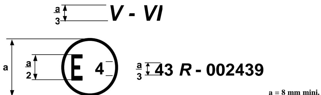
The above approval mark affixed to a double-glazed unit shows that the component concerned has been approved in the Netherlands (E 4) pursuant to Regulation No. 43 under approval No. 002439. The approval number indicates that the approval was granted in accordance with the requirements of Regulation No. 43.
