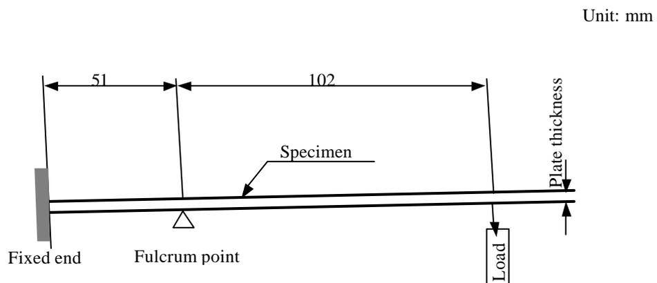
Figure 21: Method of setting up the test specimen
