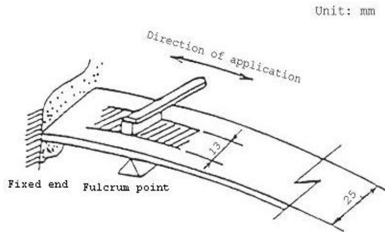
Figure 22: Method of applying chemicals to the test specimen
